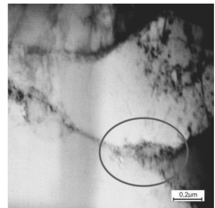
Fig. 13. The structure of CuNi25 (A) 150 after deformation at 475°C (TEM)
