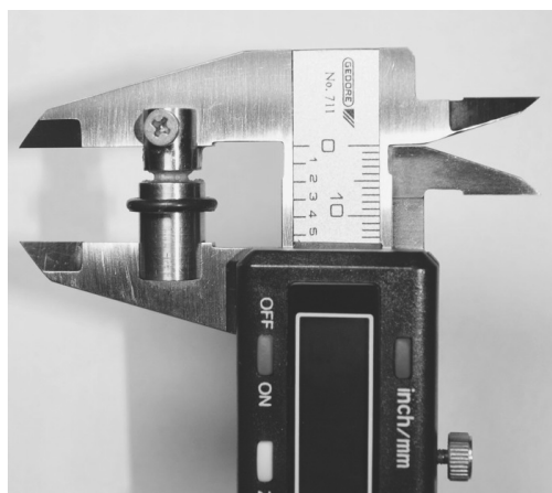
Fig. 2. Examination of extensibility of a sample of denture adhesive rarefied by artificial saliva
