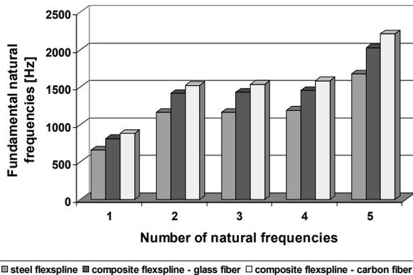
Fig. 5. Fundamental natural frequencies of a flexspline with an external flange HFUS 32-100
