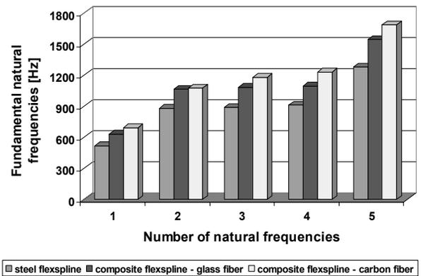
Fig. 7. Fundamental natural frequencies of a flexspline with an external flange HFUS 40-100
