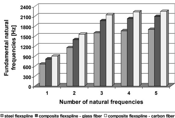
Fig. 6. Fundamental natural frequencies of a flexspline with a base HFUC 40-100
