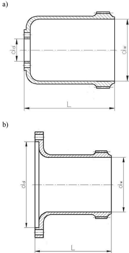
Fig. 2. Basic geometrical dimensions of the following flexsplines: a) the flexspline type HFUC, b) the flexspline type HFUS
