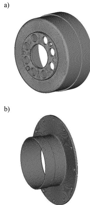
Fig. 3. Three-dimensional FEM models of flexsplines: a) featuring the HFUC base, b) featuring the HFUS external flange
