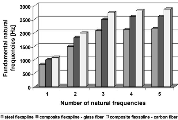
Fig. 4. Fundamental natural frequencies of a flexspline with a base HFUC 32-100
