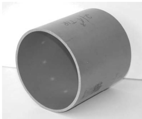
Fig. 5. Sample No. 1 after tests method for resistance to external blows by the round-the-clock method. White marks on the pipe
