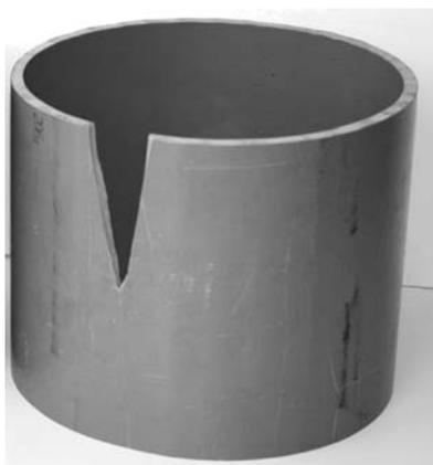
Fig. 3. Sample No. 2 after tests method for resistance to external blows by the round-the-clock method
