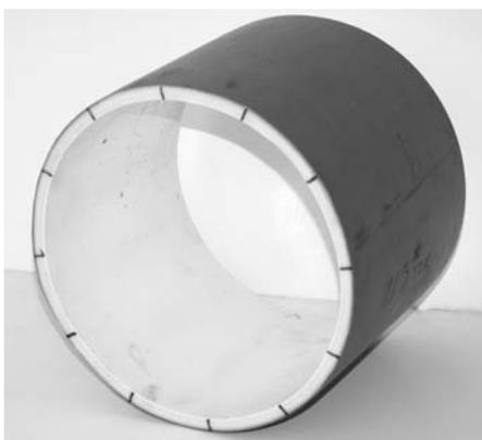
Fig. 4. Sample No. 5 after tests method for resistance to external blows by the round-the-clock method. No marks on the pipe
