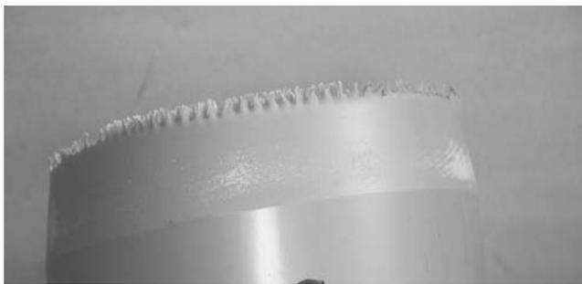
Fig. 7. Samples No.3 after immersion in dichloromethane - the best surface sample after this test
