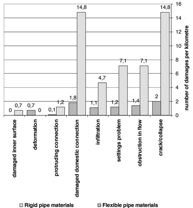
Fig. 1. Number of damages per kilometre (2006 y. in Germany) [3]
