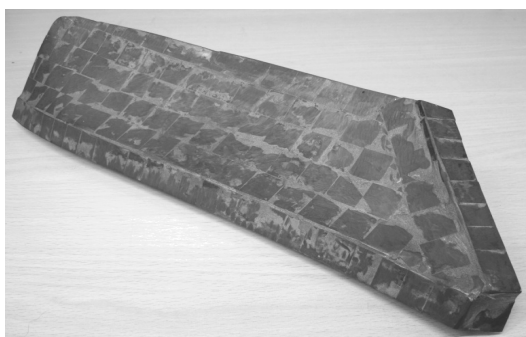
Fig. 2. View of a propeller mixer of crushed gravel with the abrasion-resisting layer of a large size surface covered with plates of cermets brazed to the base
