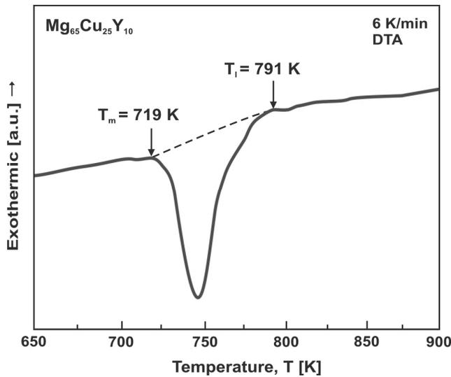
Fig. 7. DTA curve of Mg<sub>65</sub>Cu<sub>25</sub>Y<sub>10</sub> alloy as master alloy (heating rate 6 K/min)
