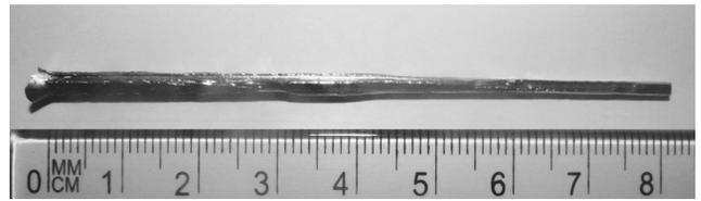
Fig. 5. Outer morphology of as-cast glassy  $Mg_{65}Cu_{25}Y_{10}$  alloy rod with diameter of 1.5 and 2 mm
