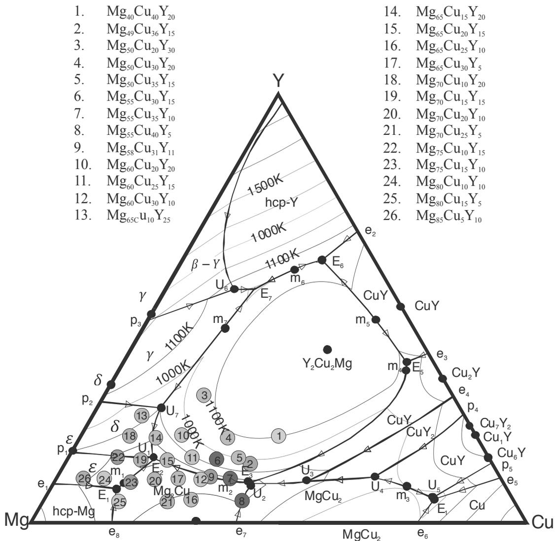
Fig. 3. Liquidus diagram of ternary Mg-Cu-Y with marked reporting composition points where fully amorphous sample was reported in literature [1-19]
