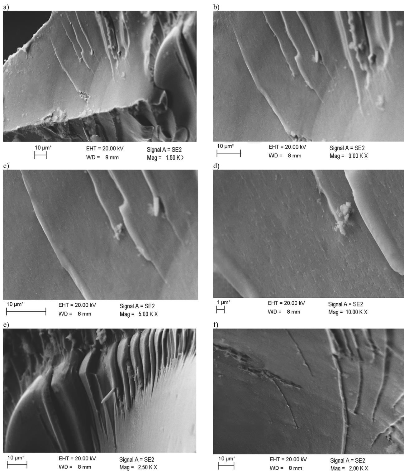
Fig. 10. SEM micrographs of the fracture surface of Mg<sub>5</sub>Cu<sub>25</sub>Y<sub>10</sub> amorphous rod in as-cast state with diameter of 2 mm (a-f)
