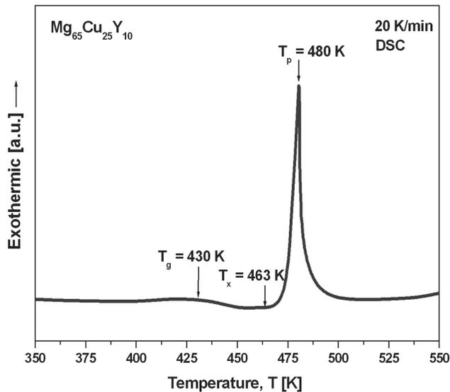
Fig. 8. DSC curves of Mg<sub>65</sub>Cu<sub>25</sub>Y<sub>10</sub> glassy alloy rod in as-cast state (heating rate 20 K/min)
