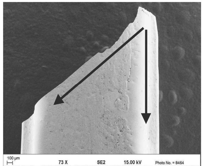
Fig. 9. Outer surface of cast glassy Mg<sub>65</sub>Cu<sub>25</sub>Y<sub>10</sub> alloy rod subjected to bending fracture
