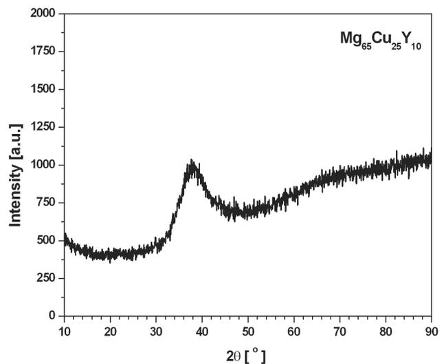
Fig. 6. X-ray diffraction pattern of  $Mg_{65}Cu_{25}Y_{10}$  glassy rod in as-cast state with diameter of 2 mm
