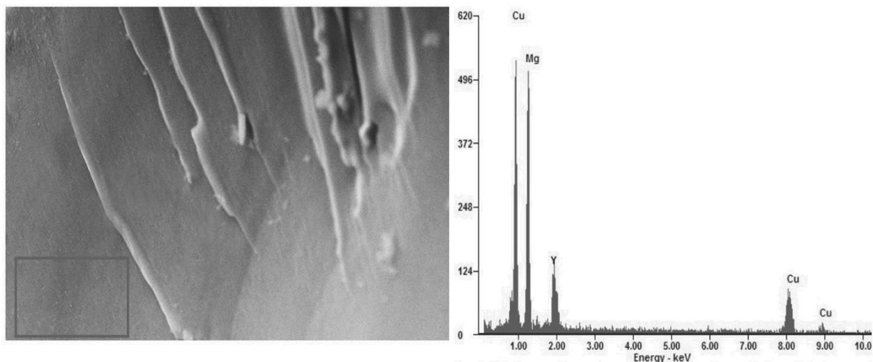
Fig. 11. SEM micrographs of  $Mg_{65}Cu_{25}Y_{10}$  amorphous rod in as-cast state with marked area for which energy dispersive X-ray analysis (EDX) was performed
