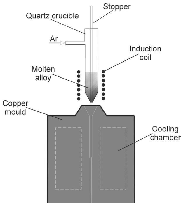
Fig. 4. Schematic illustration of the pressure die casting equipment used for casting bulk amorphous rods
