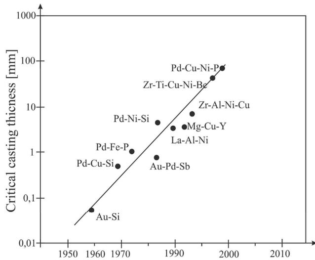
Fig. 1. Critical casting thickness for glass formation of chosen alloy systems as a function of their discovery year [3]
