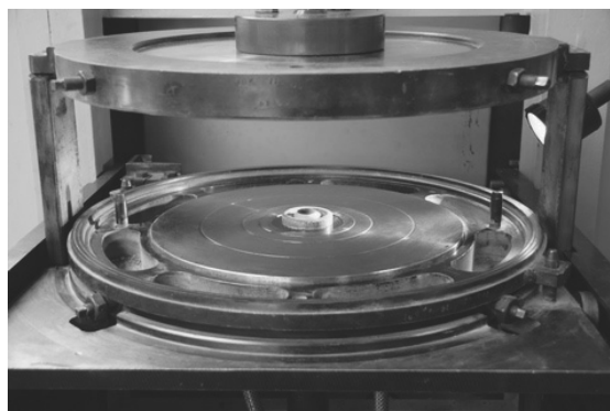
Fig. 2. Assembly for HP-HT sintering (Bridgman type apparatus)
