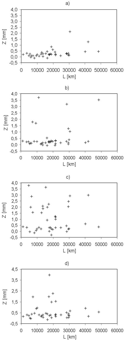
Fig. 4. Dependence of linear lift wear for angle  $\alpha = 0^\circ$  from mileage for the following cam types: a) 1 intake, b) 2 intake, c) 1 exhaust, 2 exhaust
