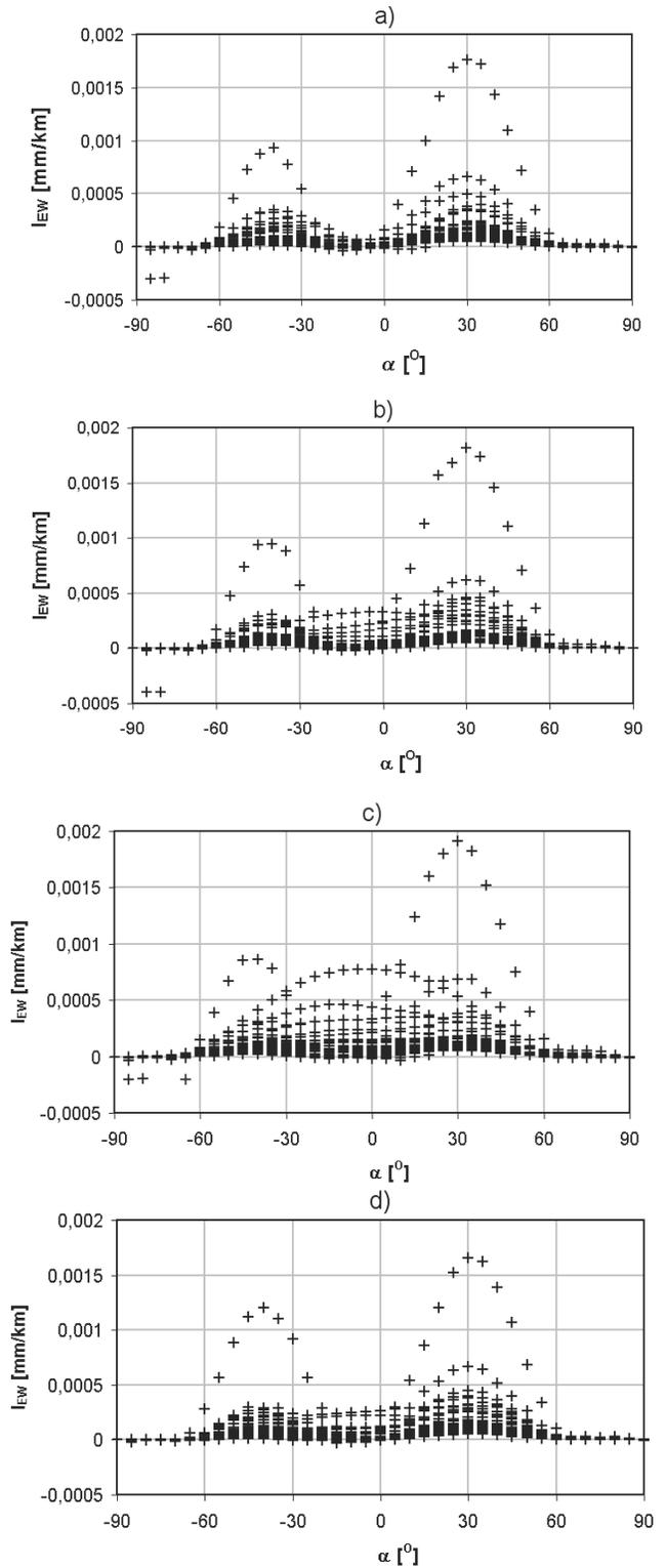
Fig. 5. Operational cam lift wear intensity in the function of angle  $\alpha$ : a) intake cam 1, b) intake cam 2, c) exhaust cam 1, d) exhaust cam 2
