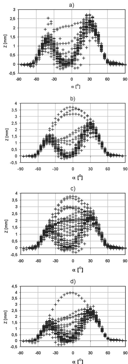
Fig. 3. Dependence of linear lift wear of the cams tested from angle  $\alpha$  for the following cam types: a) 1 intake, b) 2 intake, c) 1 exhaust, 2 exhaust
