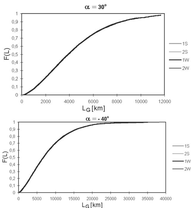
Fig. 7. Distribution functions of mileage  $L_G$  until threshold wear of 0.5 mm for:  $\alpha = -40^\circ$  and  $\alpha = 30^\circ$
