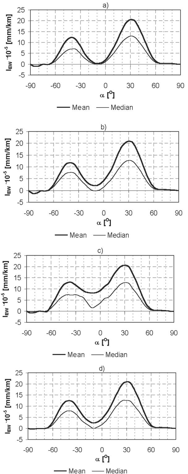
Fig. 6. Mean and median for relative operational wear intensity in the function of angle  $\alpha$ : a) intake cam 1, b) intake cam 2, c) exhaust cam 1, d) exhaust cam 2
