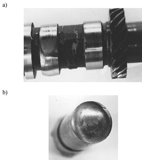
Fig. 1. Worn-out components of a cam/follower system (on car mileage of 124 km) [1]: a) camshaft with a heavily worn first cam (on the left), b) cam follower
