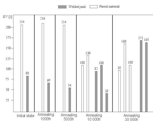
Fig. 5. Impact resistance of parent material and welded joint in initial state and after annealing at 550°C
