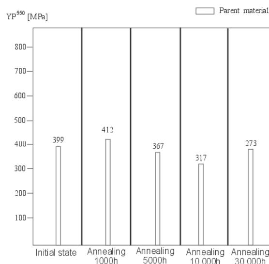
Fig. 9. Yield point at elevated temperature YP of parent material and welded joint in initial state and after annealing at 600°C
