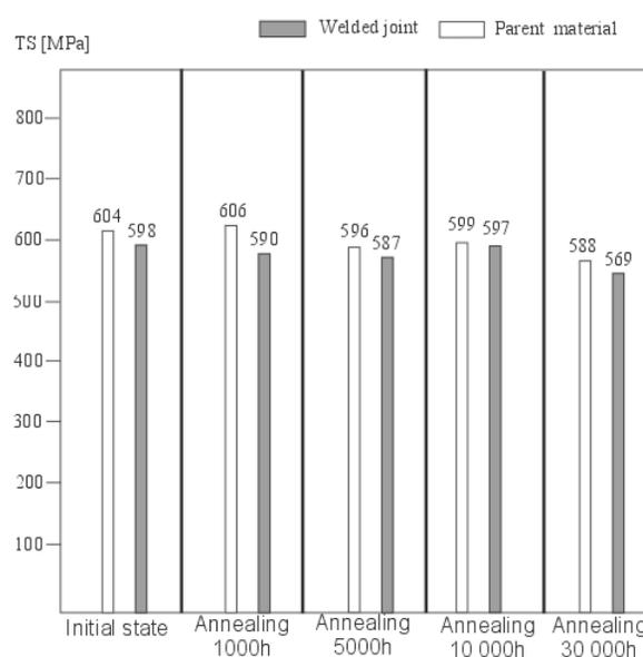
Fig. 1. Tensile strength of parent material and welded joint in initial state and after annealing at 550°C
