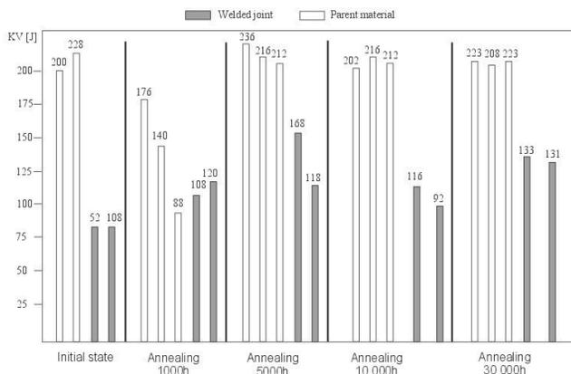
Fig. 10. Impact resistance of parent material and welded joint in initial state and after annealing at 600°C
