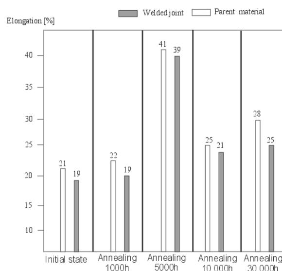
Fig. 8. Elongation  $A_5$  of parent material and welded joint in initial state and after annealing at 600°C
