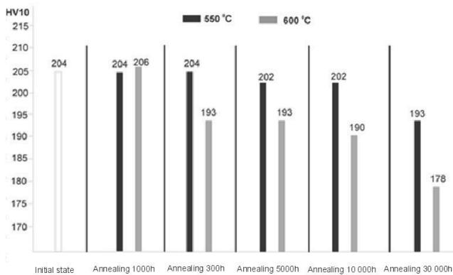
Fig. 11. Effect of long-term annealing at 550 and 600°C on hardness HV10 of 7CrMoVTiB10-10 steel
