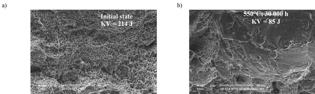
Fig. 17. Fractography of impact test samples of 7CrMoVTiB10-10 steel after long-term annealing at elevated temperature, observed under scanning electron microscope (mag. 500x): a) in initial state, b) at 550°C after 30,000 hours
