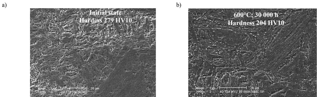
Fig. 16. Structure of weld metal of homogeneous circumferential welded joint made of 7CrMoVTiB10-10 steel after long-term annealing at elevated temperature, observed under scanning electron microscope (mag. 1000x): a) in initial state, b) at 600°C after 30,000 hours
