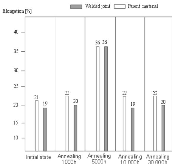
Fig. 3. Elongation A<sub>5</sub> of parent material and welded joint in initial state and after annealing at 550°C
