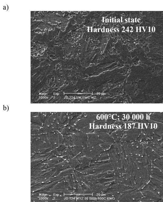
Fig. 15. Structure of heat-affected zone of homogeneous circumferential welded joint made of 7CrMoVTiB10-10 steel after long-term annealing at elevated temperature, observed under scanning electron microscope (mag. 1000x): a) in initial state, b) at 600°C after 30,000 hours
