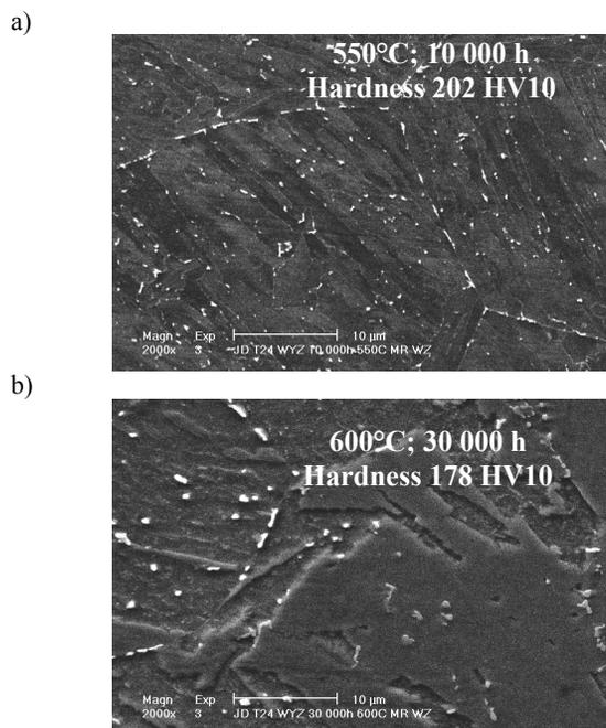
Fig. 14. Structure of 7CrMoVTiB10-10 steel after long-term annealing at elevated temperature, observed under scanning electron microscope (mag. 2000x): a) at 550°C after 10,000 hours, b) at 600°C after 30,000 hours
