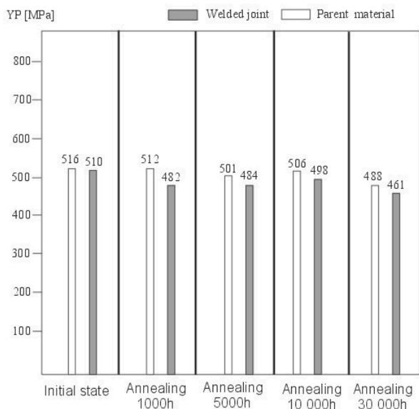
Fig. 2. Yield point of parent material and welded joint in initial state and after annealing at 550°C
