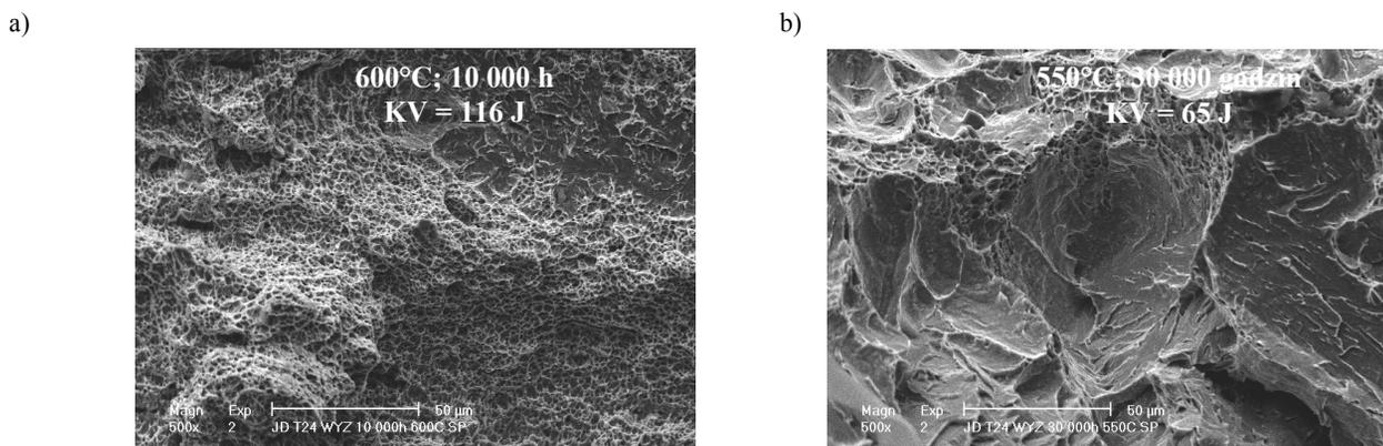
Fig. 18. Fractography of impact test samples of the weld of homogeneous circumferential welded joint made of 7CrMoVTiB10-10 steel after long-term annealing at elevated temperature, observed under scanning electron microscope (mag. 500x): a) at 600°C after 10,000 hours, b) at 550°C after 30,000 hours
