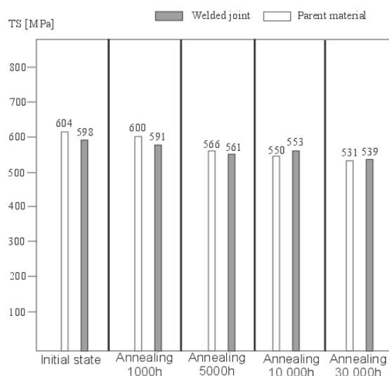
Fig. 6. Tensile strength of parent material and welded joint in initial state and after annealing at 600°C
