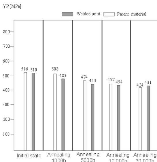
Fig. 7. Yield point of parent material and welded joint in initial state and after annealing at 600°C
