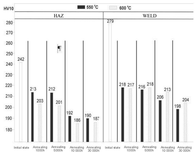
Fig. 12. Effect of long-term annealing at 550 and 600°C on hardness HV10 of heat-affected zone and weld metal of circumferential welded joint made of 7CrMoVTiB10-10 steel
