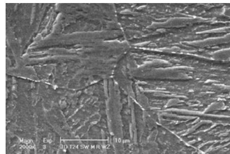
Fig. 13. Image of structure observed under scanning electron microscope, selected for testing of pipe made of low-alloy bainitic steel 7CrMoVTiB10-10 (mag. 2000x)
