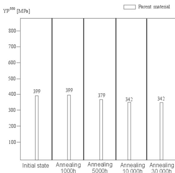
Fig. 4. Yield point at elevated temperature YP of parent material and welded joint in initial state and after annealing at 550°C
