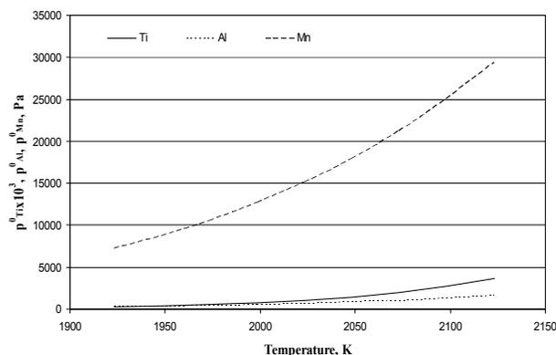
Fig. 5. Titanium, aluminium and manganese pressures over the pure component at 1923-2123 K
