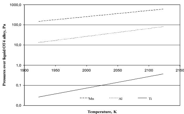
Fig. 6. Titanium, aluminium and manganese pressures over liquid OT4 alloy
