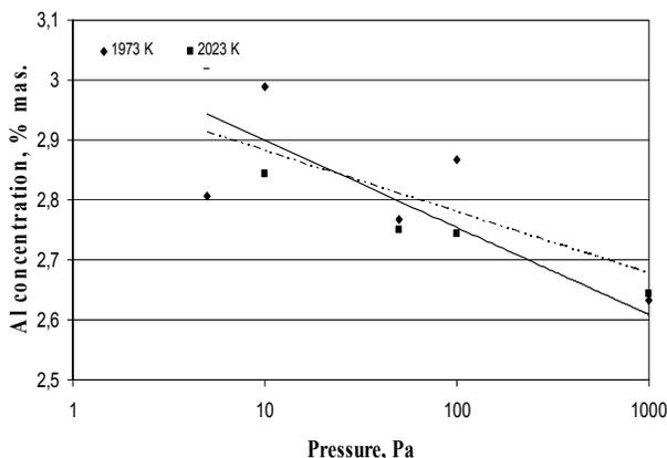
Fig. 3. Changes in the alloy Al fraction related to the VIM chamber pressure during smelting
