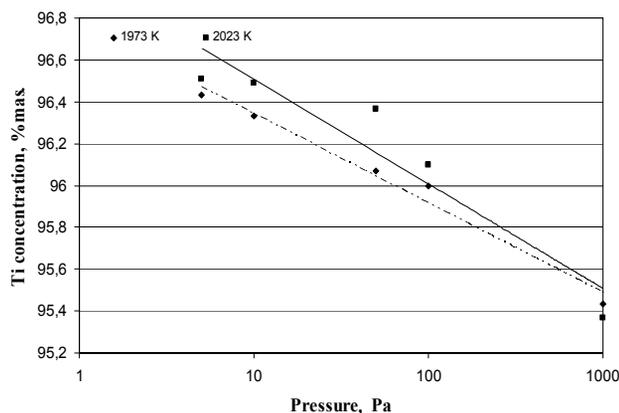
Fig. 2. Changes in the alloy Ti fraction related to the VIM chamber pressure during smelting
