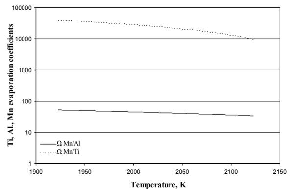
Fig. 7. Changes in the coefficient  $\Omega$  values versus temperature for the basic alloy components
