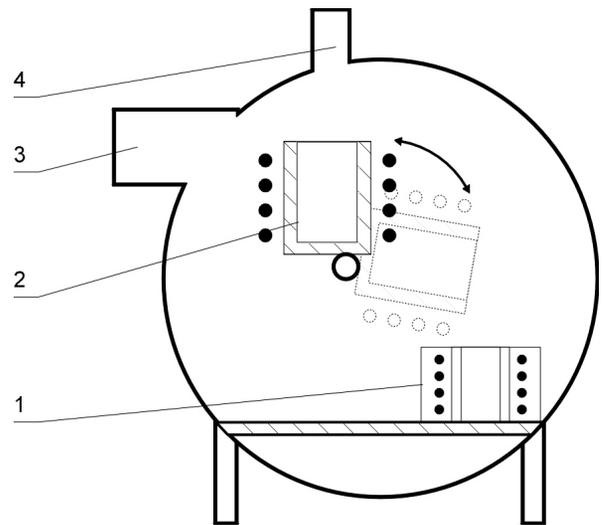
Fig. 1. The scheme of experimental device: 1 - an ingot mould with a heating system; 2 - an inductor with a ceramic melting pot; 3 - an outlet to vacuum pumps; 4 - a mounting point for the system for temperature measurements and sample collection
