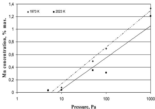
Fig. 4. Changes in the alloy Mn fraction related to the VIM chamber pressure during smelting
