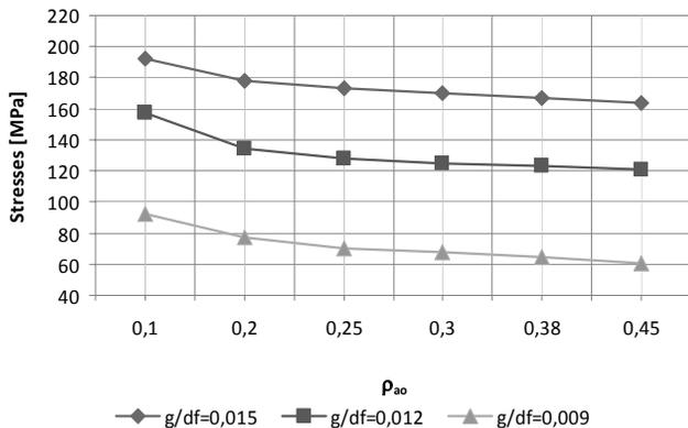
Fig. 4. The influence of the curve radius of the tool head  $\rho_{a0}$  and relative coating thickness  $g/d_f$  on value of stresses in the bottom land, with:  $w_0/m = 1$ ;  $M_{nom} = 0$
