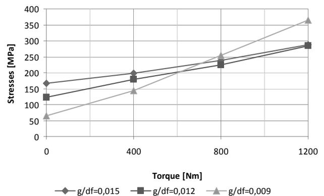
Fig. 6. The influence of the torque and relative coating thickness  $g/d_f$  on value of stresses in the bottom land of a tooth, with:  $\rho_{a0} = 0.38$ ;  $w_0/m = 1$
