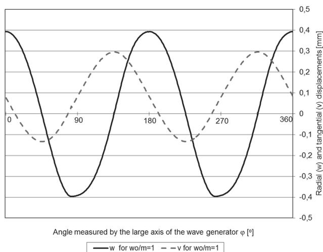
Fig. 1. Chart of radial ( $w$ ) and tangential ( $v$ ) displacements as a function of angle measured from the large axis of the wave generator
