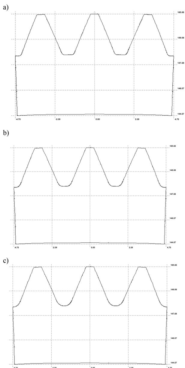
Fig. 8. The contours of the toothed ring generated by tooth profile generator for: a)  $\rho_{a0} = 0.1$ ; b)  $\rho_{a0} = 0.25$ ; c)  $\rho_{a0} = 0.38$
