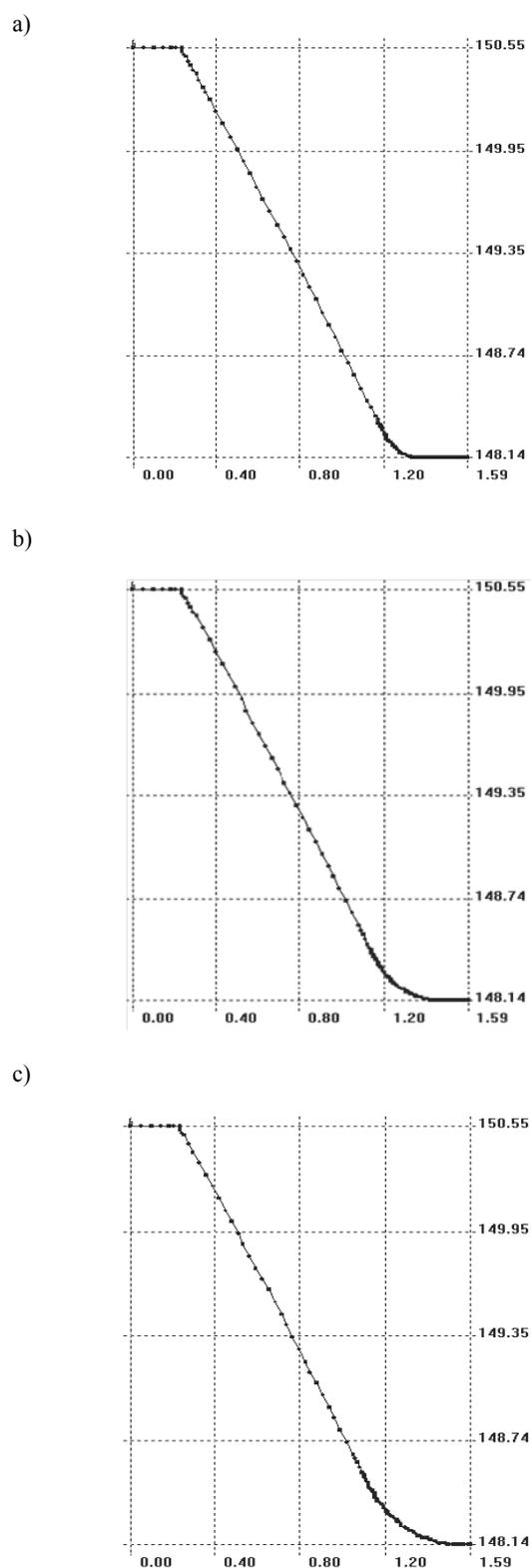
Fig. 7. The lateral contour lines of the tooth generated by tooth profile generator for: a)  $\rho_{a0} = 0.1$ ; b)  $\rho_{a0} = 0.25$ ; c)  $\rho_{a0} = 0.38$
