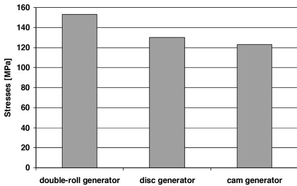
Fig. 3. The maximum value of stress in the bottom land of a tooth, depending on the type of wave generator with:  $g/d_f = 0.012$ ;  $w_0/m = 1$ ;  $M_{nom} = 0$
