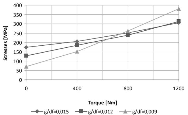
Fig. 5. The influence of the torque and relative coating thickness  $g/d_f$  on value of stresses in the bottom land of a tooth, with:  $\rho_{a0} = 0.25$ ;  $w_0/m = 1$
