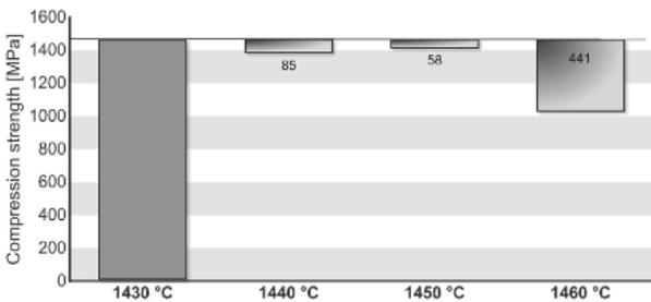
Fig. 15. Influence of casting temperature on compression strength of the Remanium 2000+ alloy
