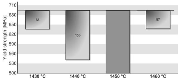
Fig. 14. Influence of casting temperature on yield strength of the Wirobond LFC alloy
