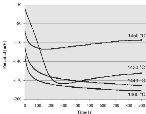
Fig. 6. Open circuit potential curves after 900s tests for Wirobond LFC
