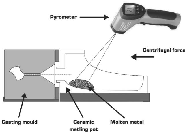
Fig. 2. Centrifugal casting machine with measurement temperature of the melted alloy [9]
