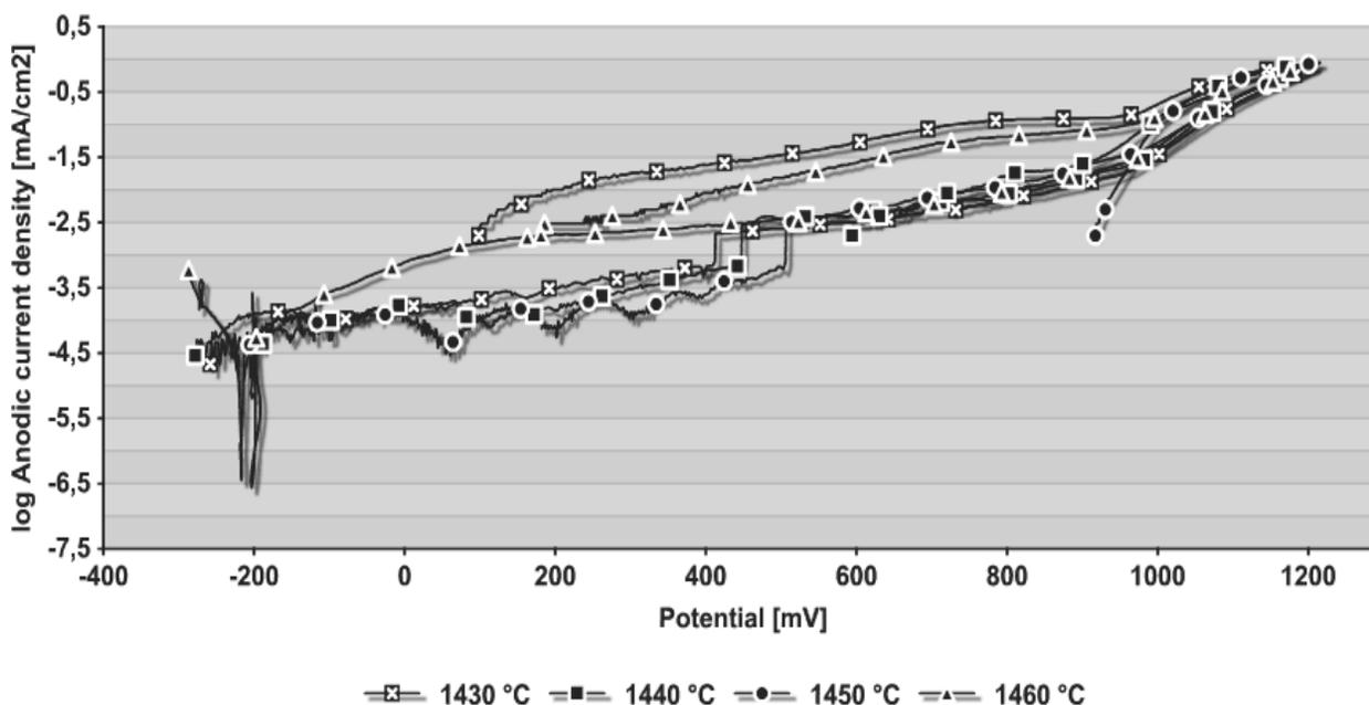
Fig. 8. Potentiodynamic curves of pitting corrosion Wirobond LFC alloy after four different casting temperature
