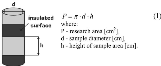
Fig. 3. Sample prepared to electrochemical test
