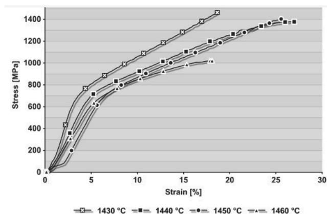
Fig. 11. Compression strength curves after different casting of the Remanium 2000+ alloy
