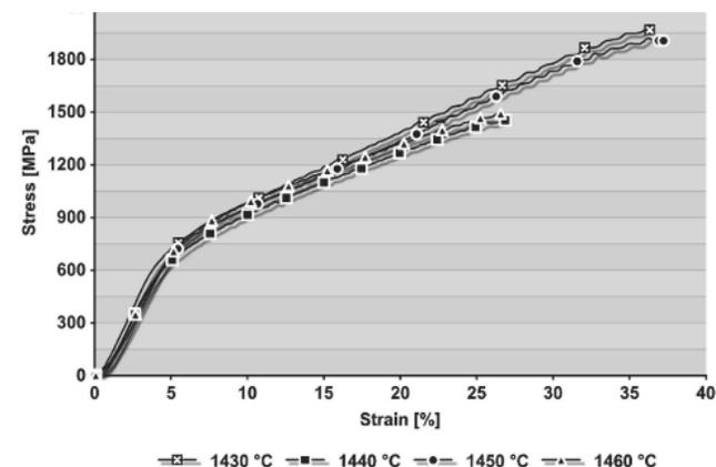
Fig. 12. Compression strength curves after different casting of the Wirobond LFC alloy
