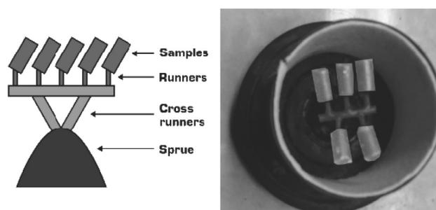
Fig. 1. The prepared model and mould to casting
