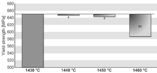
Fig. 13. Influence of casting temperature on yield strength of the Remanium 2000+ alloy
