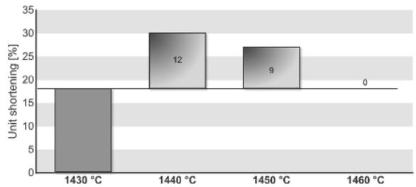
Fig. 17. Influence of casting temperature on shortening of the Remanium 2000+ alloy
