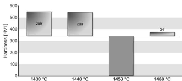
Fig. 10. Influence of casting temperature on hardness of the Wirobond LFC alloy
