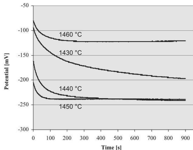
Fig. 5. Open circuit potential curves after 900s tests for Remanium 2000+
