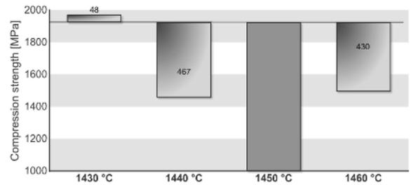
Fig. 16. Influence of casting temperature on compression strength of the Wirobond LFC alloy
