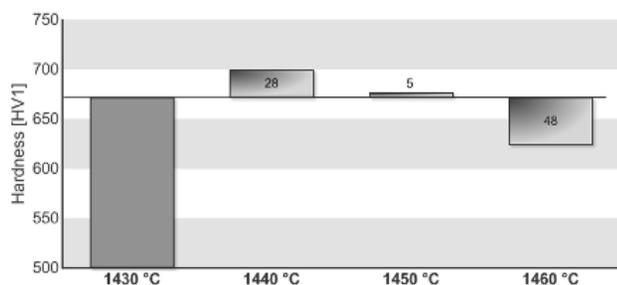
Fig. 9. Influence of casting temperature on hardness of the Remanium 2000+ alloy
