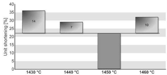
Fig. 18. Influence of casting temperature on shortening of the Wirobond LFC alloy
