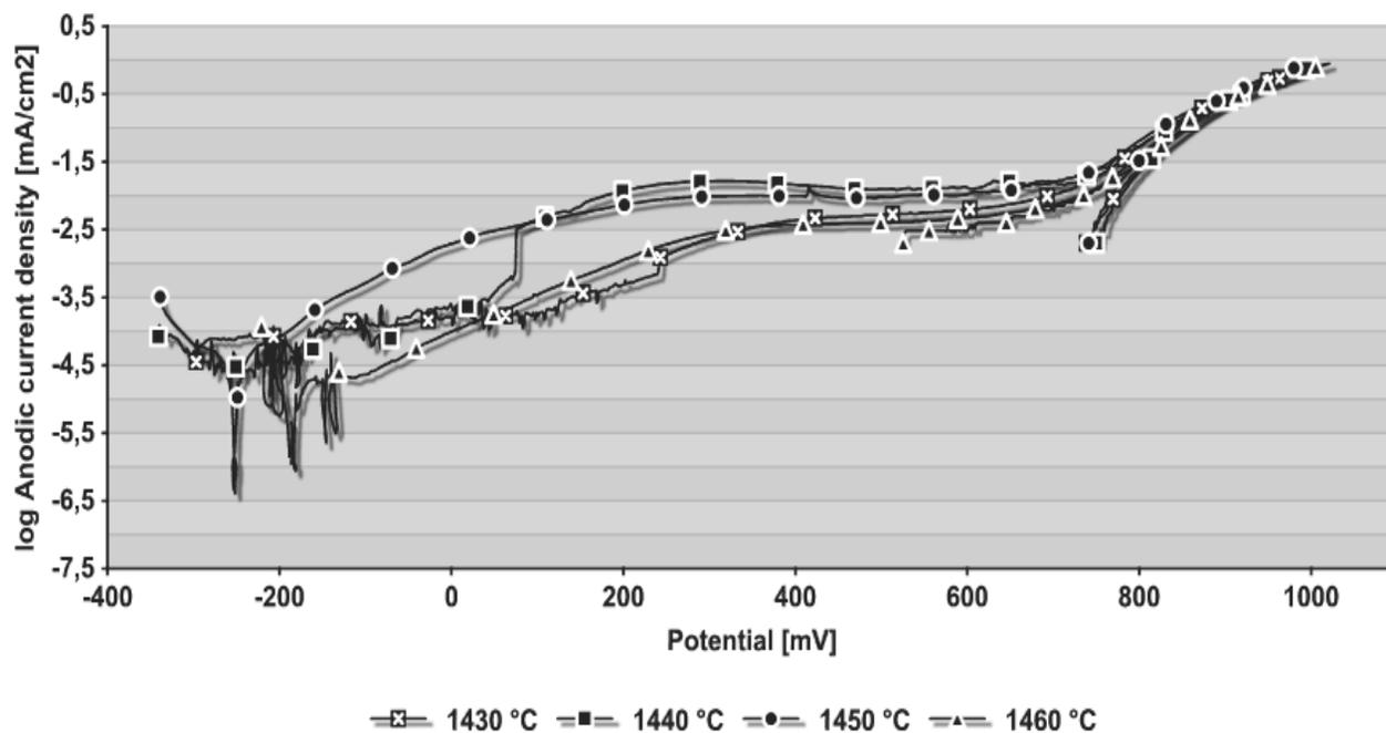
Fig. 7. Potentiodynamic curves of pitting corrosion Remanium 2000+ alloy after four different casting temperature
