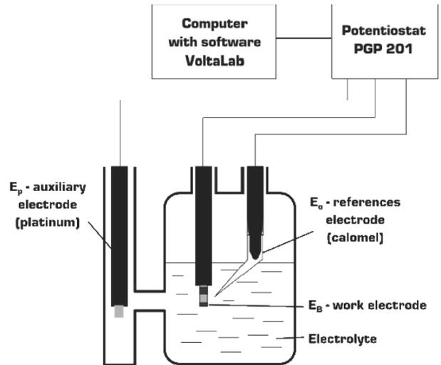
Fig. 4. Scheme of the corrosion resistance set to evaluate pitting resistance
