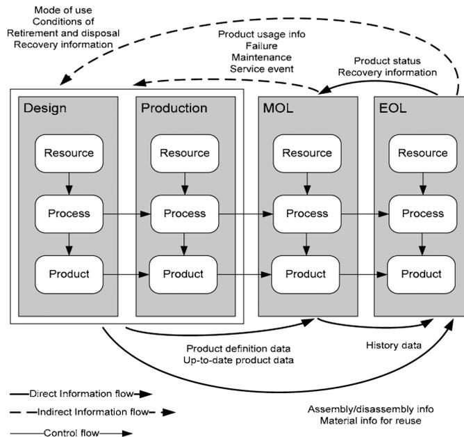
Fig. 1. Information flow between the different stages of PLM
