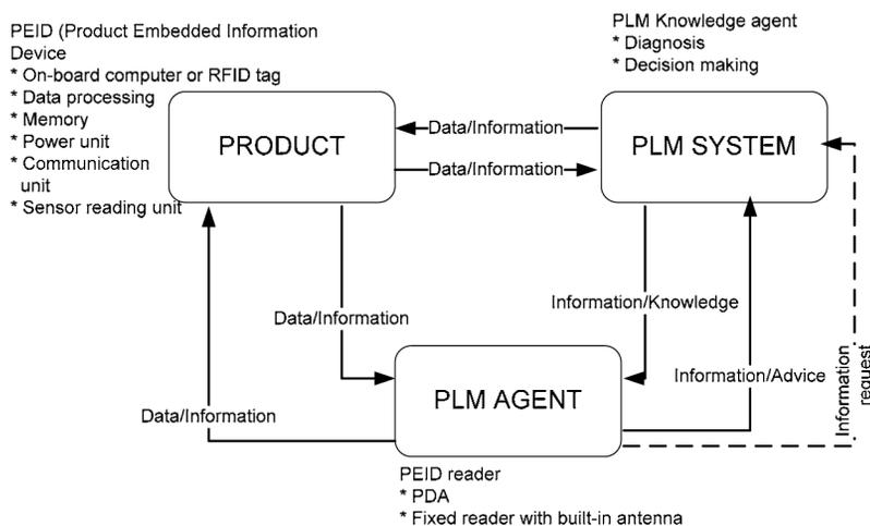
Fig. 2. Concept of closed-loop PLM
