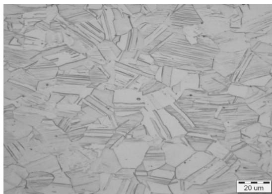
Fig. 17. Microstructure of CuSn6 strip deformed after 4 passes of RCS process, perpendicular to the rolling direction
