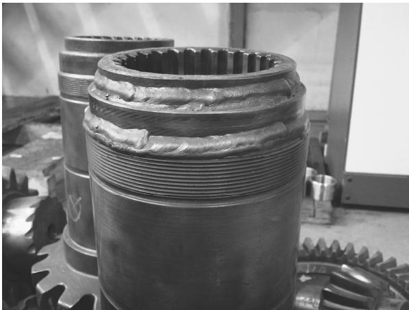
Fig. 6. Shaft after surface welding
