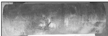
Fig. 1. Material for investigations in the form of 14MoV6-3 (13HMF) steel homogeneous circumferential welded joint of primary steam pipeline after 200,000 h service
