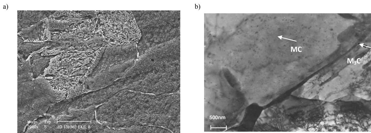
Fig. 4. Ferritic-bainitic structure of 14MoV6-3 steel in initial state a) SEM, b) TEM
