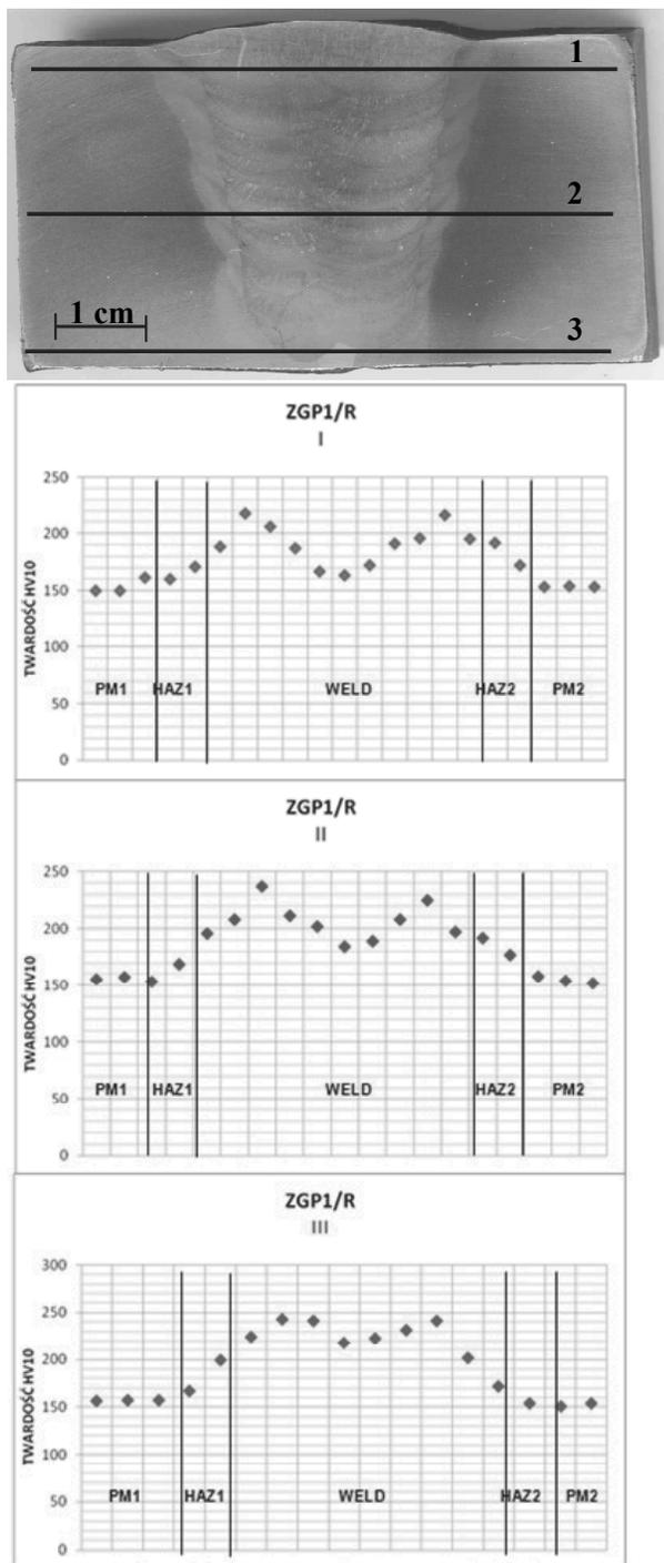
Fig. 10. Results of hardness tests of 14MoV6-3 steel primary steam pipeline welded joint. Testing area - transverse microsection marked as ZGP1/R. a) from the face side, b) in the middle of weld, c) from the root side
