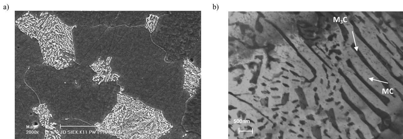
Fig. 3. Ferritic-pearlitic structure of 13CrMo4-5 steel in initial state a) SEM, b) TEM
