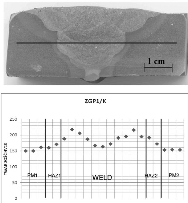
Fig. 11. Results of hardness tests of 13CrMo4-5 steel II° secondary steam superheater header welded joint. Testing area - transverse microsection marked as ZGP1/K.
