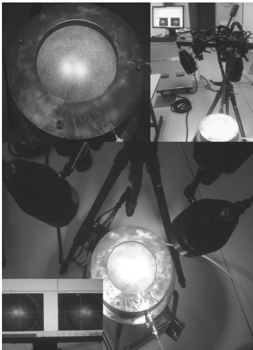
Fig. 14. Setup of the bulge tests with the GOM-ARAMIS
