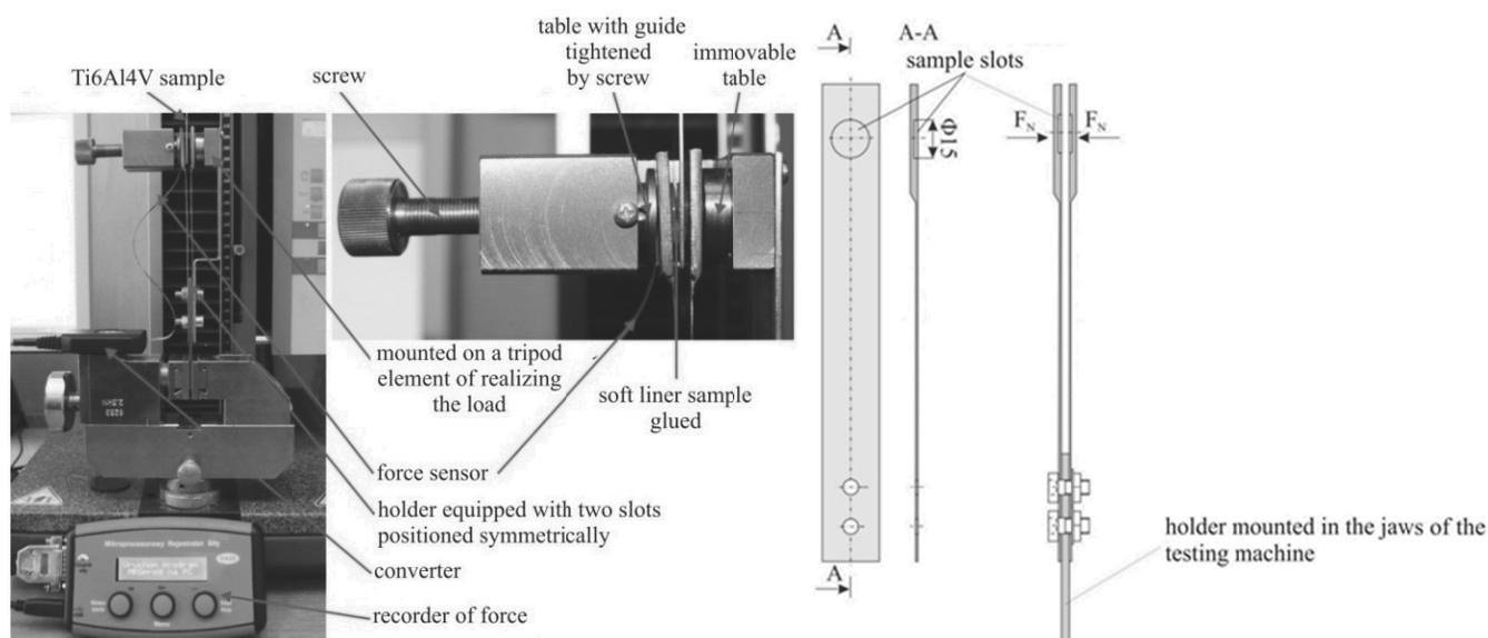
Fig. 1. A handle to test coefficient of frictions fixed in the jaws of the testing machine together with the element realizing the load and the handle scheme
