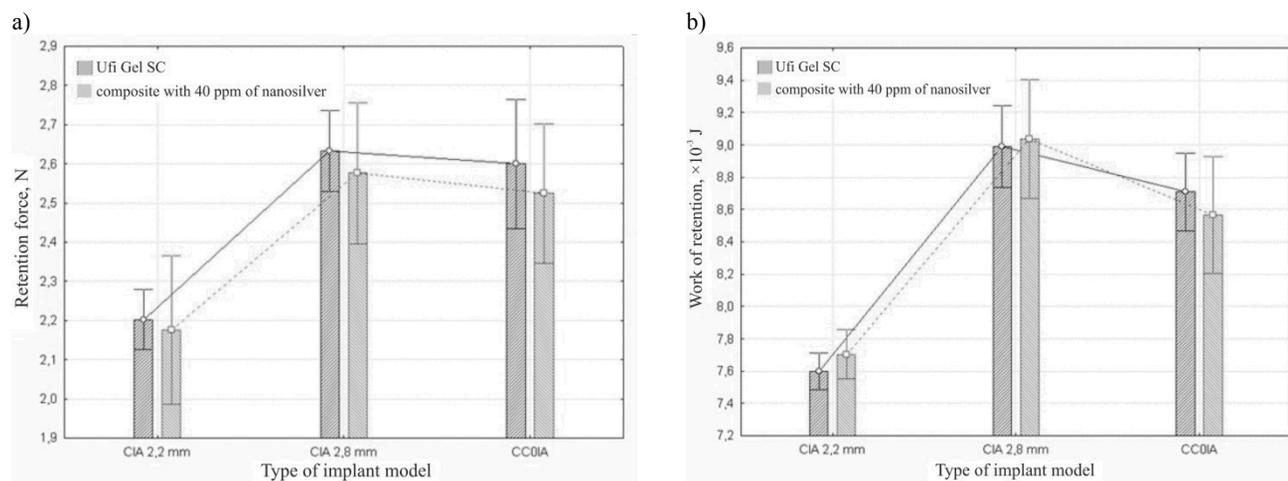
Fig. 5. A selection of the results of studies of retention forces (a) and retention works (b) obtained for elastic friction attachments made of UG material and nanocomposite with a nanosilver mass content of 40 ppm using different implant models. Confidence interval was indicated using markers
