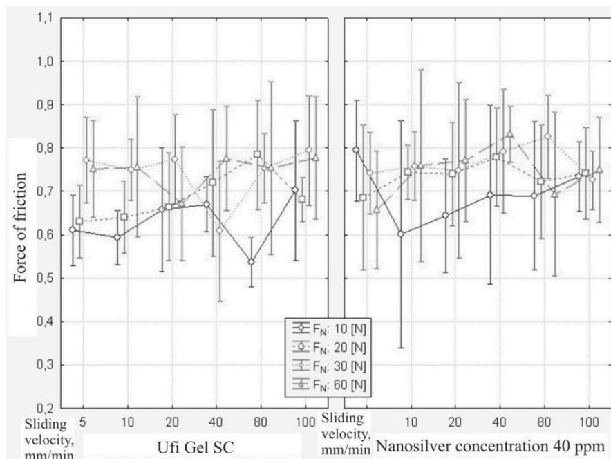
Fig. 4. A selection of coefficient of frictions obtained for samples made of UG material and nanocomposite with a nanosilver mass content of 40 ppm (in the presence of saliva) in the function of relative velocity of friction elements for four different pressure force values. Confidence interval was indicated with markers.
