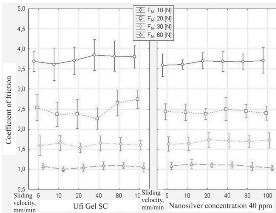
Fig. 3. A selection of coefficient of frictions obtained for samples made of UG material and nanocomposite with mass content of nanosilver of 40 ppm (without saliva) in the function of relative velocity of friction elements for four different pressure force values. Confidence interval was indicated with markers
