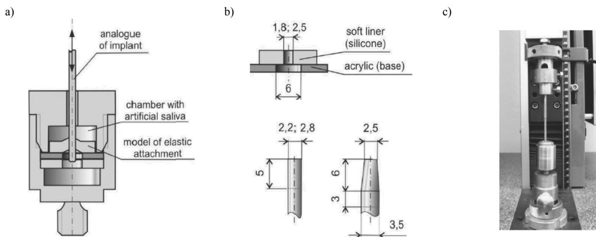
Fig. 2. The scheme of the handle used in the studies of retention characteristics of friction attachments (a), geometry and important (from the point of view of conducted experiment) dimensions of samples imitating implants and elastic models of retention elements (b), as well as the handle fixed in the testing machine during the experiment (c)
