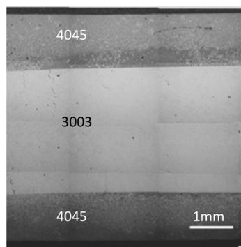
Fig. 5. Cross section of three layers clad strip
