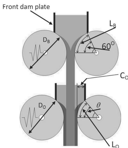
Fig. 9. Schematic illustration showing the Clearance  $C_o$  and position of the front dam plate  $\theta$ , roll diameter  $D_B$  and  $D_O$ , solidification length  $L_B$  and  $L_O$ .
