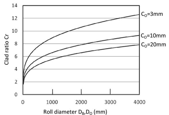
Fig. 10. Relationship among roll diameter, front dam clearance  $C_o$  and clad ratio Cr. The roll diameter  $D_B$  and  $D_O$  is same. The front dam plate of the upper roll caster for base strip is 60°
