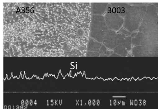
Fig. 18. Line analysis of Si around the interface between the A356 strip and 3003 strip of clad strip shown in Fig. 17
