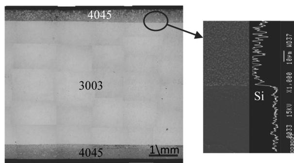
Fig. 3. Cross section of the three layers clad strip and result of the line analysis of Si around the interface
