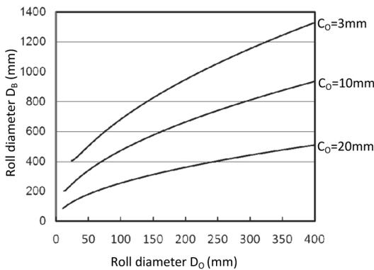
Fig. 12. Relationship among the front dam clearance  $C_o$ , roll diameter  $D_B$  and  $D_o$ . Clad ratio  $Cr$  is 8
