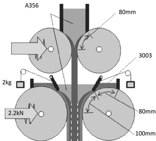
Fig. 16. Schematic illustration showing the vertical type tandem twin roll caster equipped with scrapers to cast five layers clad strip which base strip has lower melting point than that of the overlay strip
