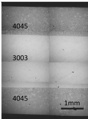
Fig. 7. Cross section of the as-cast three layers clad strip. Casting temperature 700°C of melt of 4045 overlay strip was higher than the liquidus line 655°C of base strip 3003. Roll speed was 30 m/min
