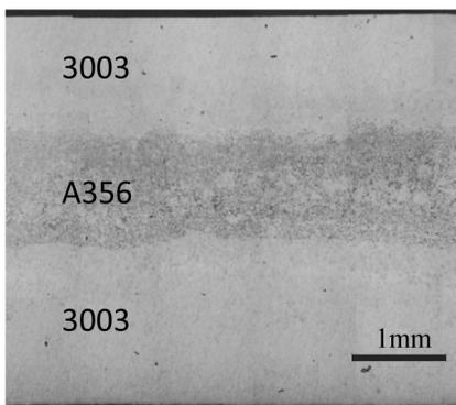
Fig. 15. Cross section of the three layers clad strip cast by the twin roll caster of Fig. 13
