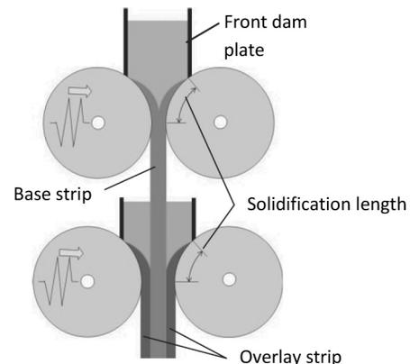
Fig. 1. Schematic illustration of a vertical type tandem twin roll caster
