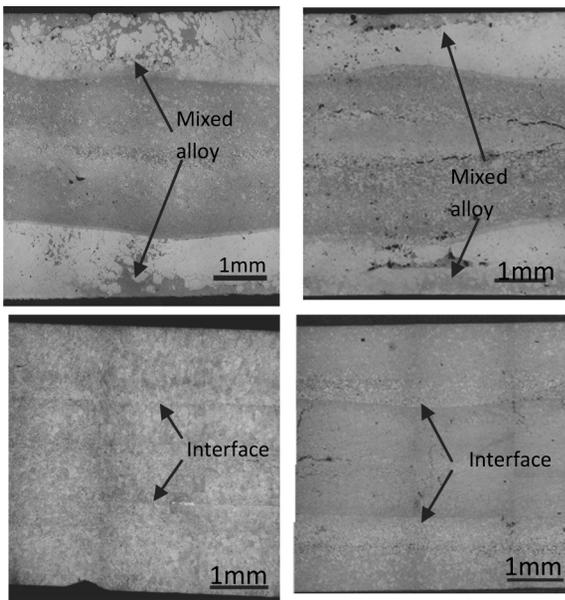
Fig. 6. Cross section of the three layers clad strip cast by the twin roll caster of Fig. 1
