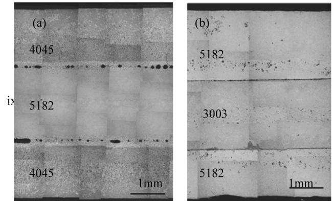
Fig. 8. Cross section as-cast three layers clad strip. Casting temperature is as below, 4045:610°C, 5182:650°C, 3003:670°C. Roll speed was 30 m/min
