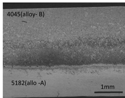
Fig. 20. Cross section of as-cast clad strip cast using the twin roll caster of Fig. 19
