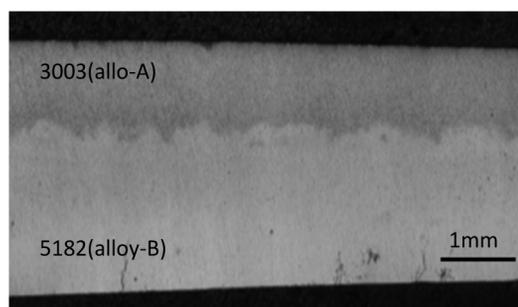
Fig. 22. Cross section of as-cast two layers clad strip cast using the twin roll caster of Fig. 19
