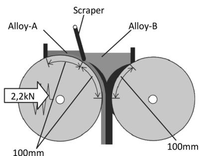
Fig. 19. Schematic illustration of a twin roll caster equipped with a scraper
