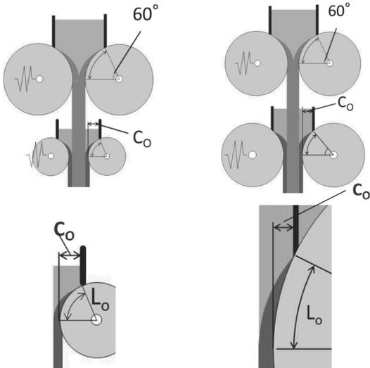
Fig. 11. Schematic illustration showing the relationship between the solidification length  $L_o$  and front dam clearance  $C_o$
