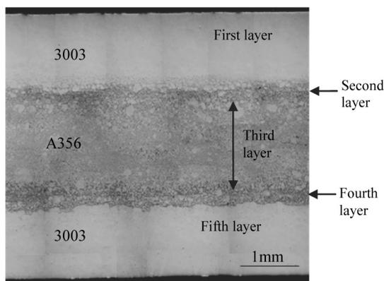
Fig. 17. Cross section of as-cast five layers clad strip cast by the twin roll caster of Fig. 16
