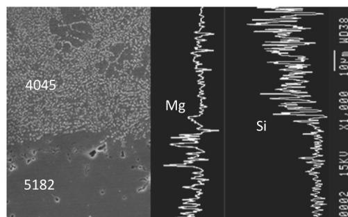
Fig. 21. SEM image and result of line analysis around the interface between the 5182 and 4045 strip
