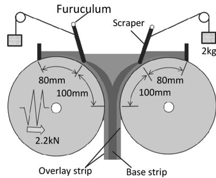
Fig. 13. Schematic illustration showing a twin roll caster equipped with scrapers
