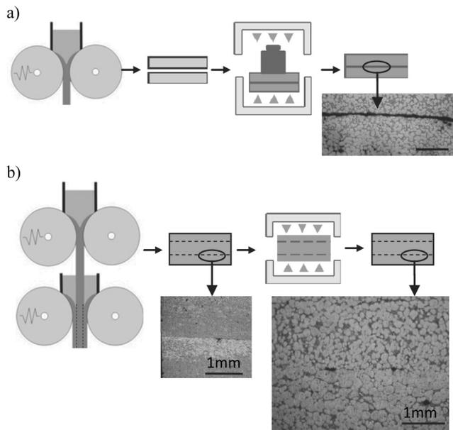
Fig. 2. Comparison of the condition of the oxide film between the surface of the single strip cast by VHSTRC and interface of the strips of the three layers clad strip cast by the VTTRC. Used alloy was A356 aluminium alloy; a) Stacked single strips of A356 alloy were heated up to 580°C for one hour. The strips were not connected; b) Three layers clad strip of A356 alloy was heated up to 580°C for one hour. Interface between the strips was not clear
