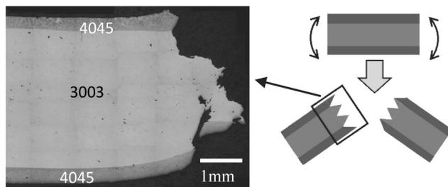
Fig. 4. Cross section of as-cast strip broken by the continuous bending
