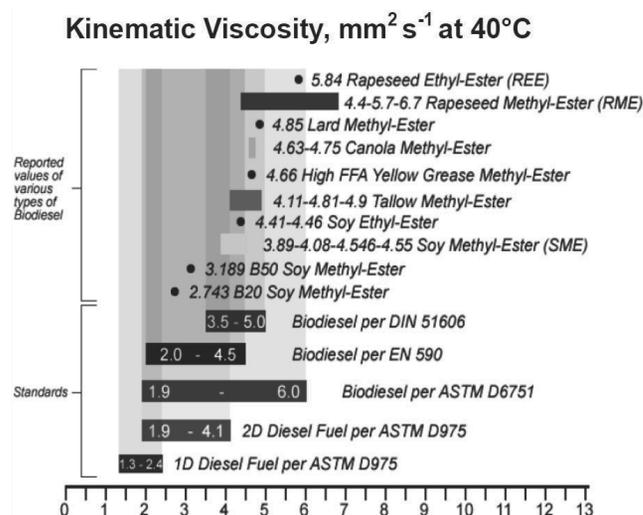
Fig. 1. Chart of the kinematic viscosity for various petroleum-based diesel and biodiesel fuel standards along with a sample of reported measurements for various types of biodiesel [11]
