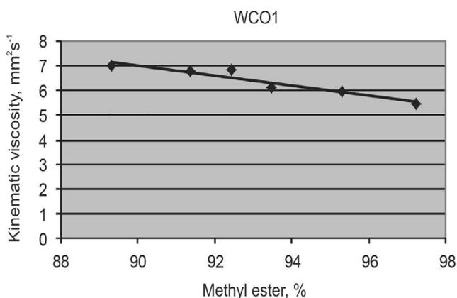
Fig. 3. The influence of methyl esters content on kinematic viscosity of produced biodiesels from waste cooking oil WCO1 and crude rapeseed oil blends
