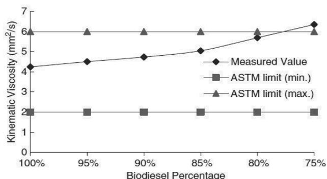
Fig. 2. Effect of raw oil presence in biodiesel on kinematic viscosity [13]
