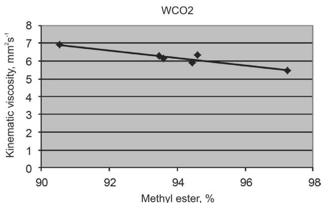
Fig. 4. The influence of methyl esters content on kinematic viscosity of produced biodiesel from waste cooking oil WCO2 and crude rapeseed oil blends
