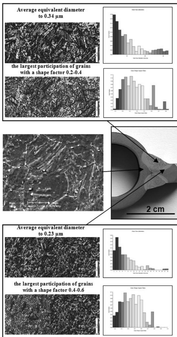
Fig. 6. Researches in the scanning electron microscope by the use of EBSD technique of the distribution of the average equivalent to the diameter of grain and the distribution of a grain shape of selected elements of the welded joint of membrane walls of the evaporator collector with supercritical working parameters made of 7CrMoVTiB10-10 steel
