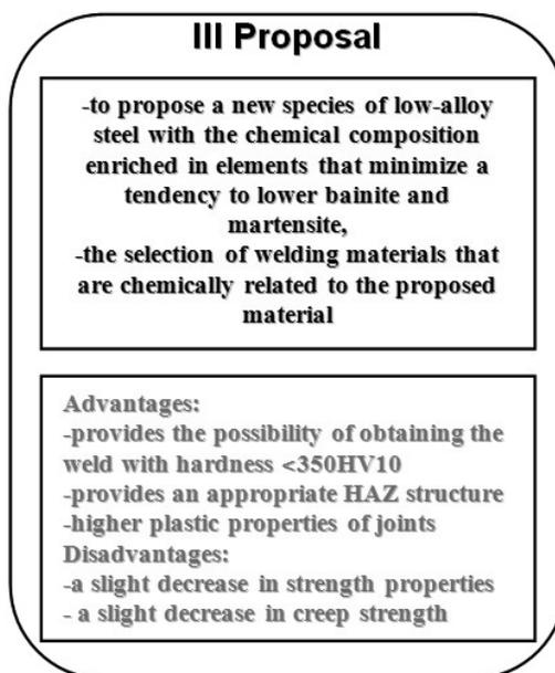
Fig. 13. Proposal of the application of a new use of new species of low-alloy steel with the chemical composition enriched in elements that minimize a tendency to lower bainite and martensite
