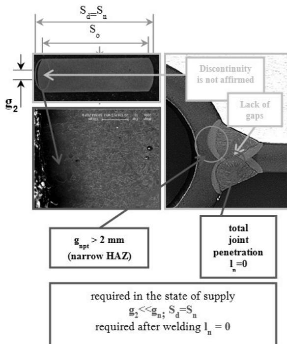
Fig. 3. The influence of the shape of the side surface in the form of a metallurgical product made in the exact required size ( $S_n = S_d$ ) on the form the weld microstructure, the participation of the heat affected zone and the size of the unmelted gap of fillet welded joints of gas-tight water walls made of 7CrMoVTiB10-10 steel  $S_n$ -nominal width,  $S_d$ -exact width,  $S_o$ -segment parallel to a flat bar width,  $g_n$  - nominal thickness;  $g_2$ -width of a contact plane with a tube
