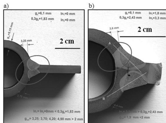
Fig. 8. Examples of obtained size of the unmelted gap between the tube and the flat bar  $l_n$  and unmelted thickness of the tube  $g_{npt}$  thickness of fillet welded joints of gas-tight water walls made of 7CrMoVTiB10-10 steel, depending on real conditions and welding parameters:
