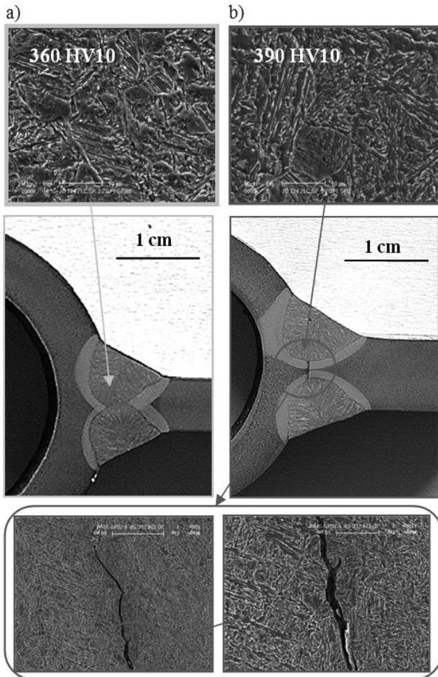
Fig. 9. Comparison of crack sensibility of obtained fillet welded joints of gas-tight water walls made of 7CrMoVTiB10-10 steel with various degrees of joint penetration of various sizes of HAZ and various forms of martensite of weld material
