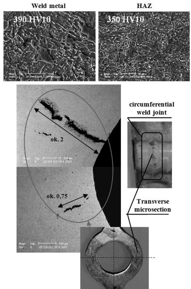
Fig. 10. Cracks in the peripheral welds of welded joints of the inner surface side in the direction perpendicular to the tube axis of the gas-tight tubular wall of 7CrMoVTiB10-10 steel
