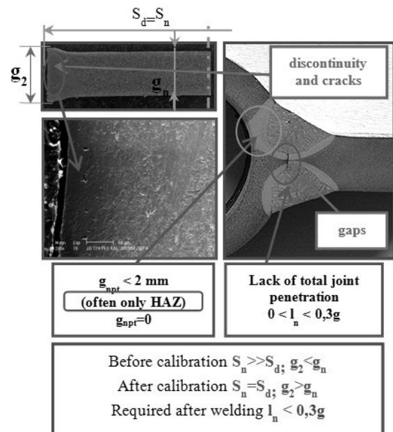
Fig. 2. The influence of the shape of the flat bar side surface in the form of steel product after the calibration prior to welding ( $S_n \neq S_d$ ) in the form of weld microstructure, the participation of the heat affected zone and the size of the gap of an unmelted crack of fillet welded joints of gas-tight water walls made of 7CrMoVTiB10-10 steel.  $S_n$  - nominal width ,  $S_d$  - exact width ,  $g_n$  - nominal thickness ;  $g_2$  - width of a contact plane with a tube
