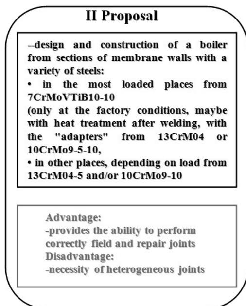
Fig. 12. Proposal of the application of tubes and flat bars made of 7CrMoVTiB10-10 steel on segments of membrane wall made only at the factory with "adapters" 13CrMo4-5 and/or 10CrMo9-10 steel for field assembly. In other places, depending on the load segments made of 13CrMo4-5 and/or 10CrMo9-10 steel
