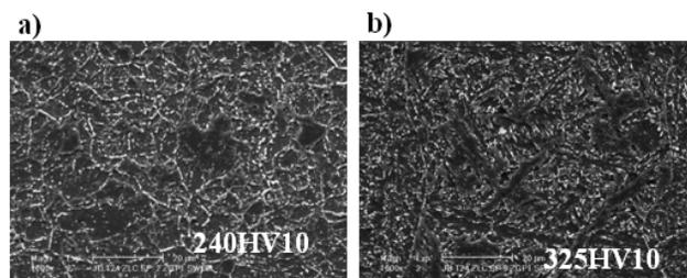
Fig. 7 The types of microstructure of the heat affected zone of welded joints in gas-tight welds of water walls made of 7CrMoVTiB10-10 steel, depending on the temperature of preheating before welding and after welding cooling speed
