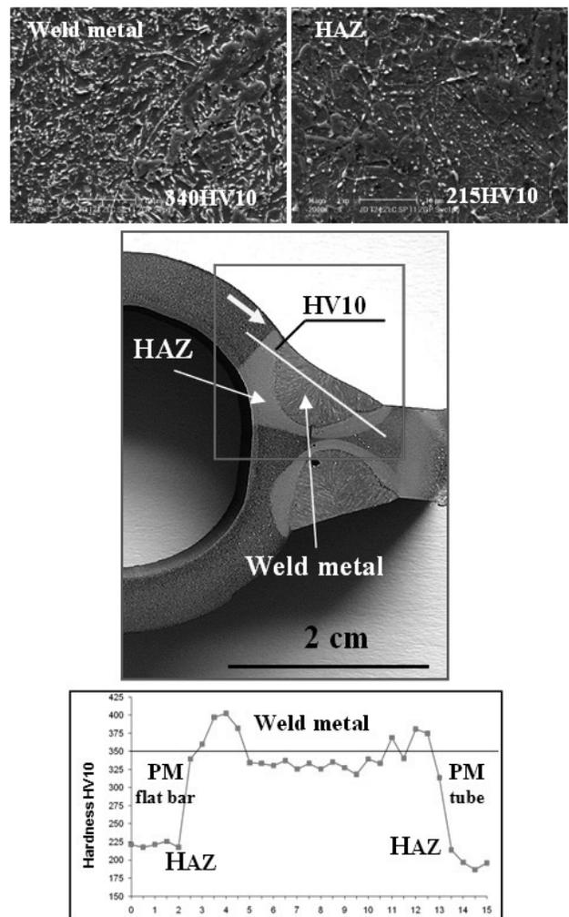
Fig. 5. The microstructure of the heat affected zone and the weld and hardness distribution in the cross section of the fillet welded joints of gas-tight water walls made of 7CrMoVTiB10-10 steel with HAZ including entire thickness of the tube (S)
