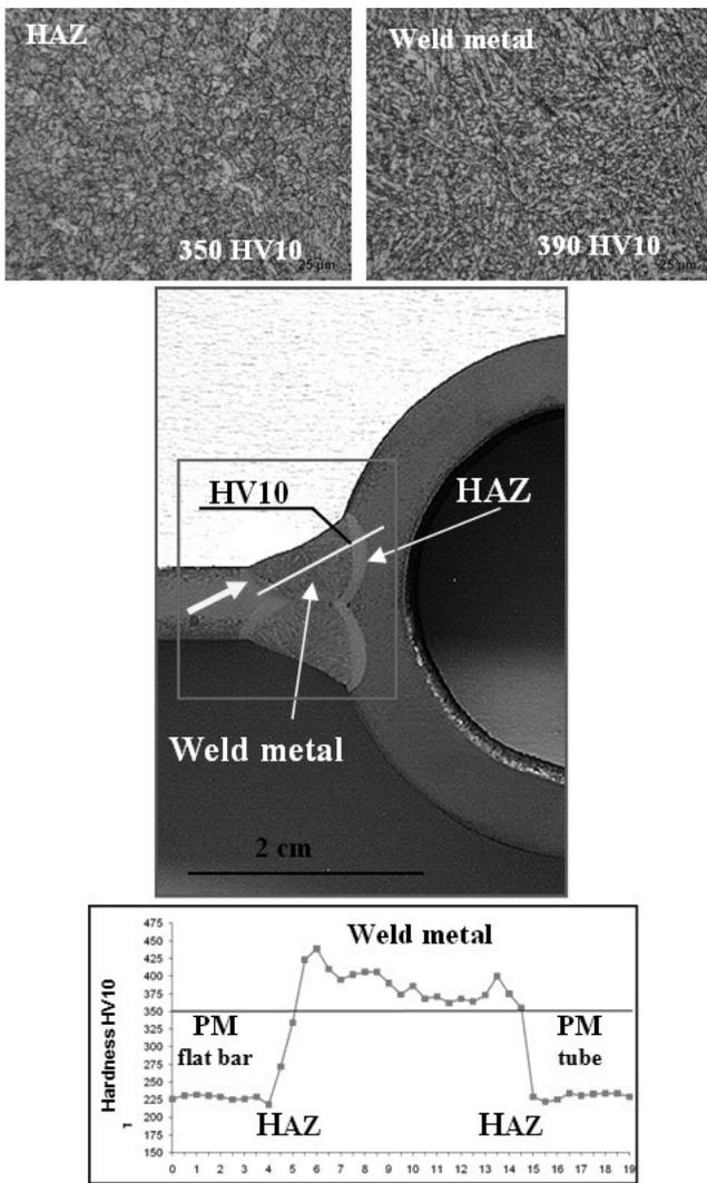
Fig. 4. The microstructure of the heat affected zone and the weld and hardness distribution in the cross section of the fillet welded joint of gas-tight water walls made of 7CrMoVTiB10-10 steel with a narrow HAZ (LM)
