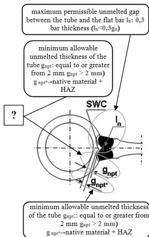
Fig. 1. Requirements for fillet welded joints of gas-tight water walls of low-alloy bainitic steels:  $S_n$  - nominal width,  $S_d$  - exact width
