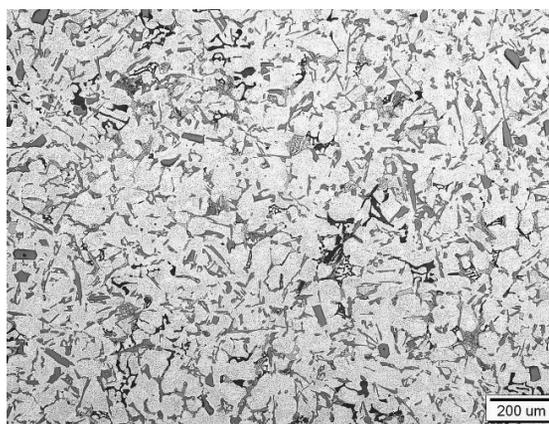
Fig. 3. Microstructure of the AC-AlSi12CuNiMg cooled with  $0.18^\circ\text{C/s}$ , with addition of Ag
