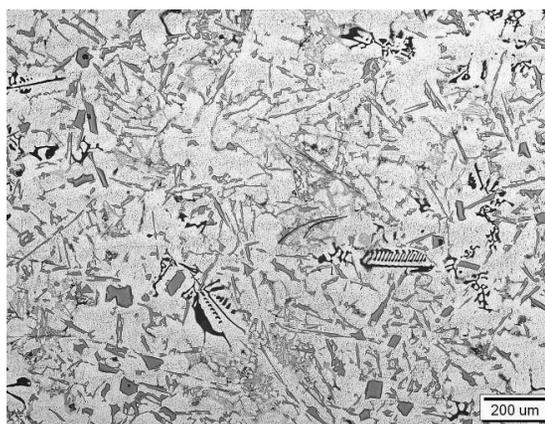
Fig. 2. Microstructure of the AC-AlSi12CuNiMg cooled with  $0.11^\circ\text{C/s}$
