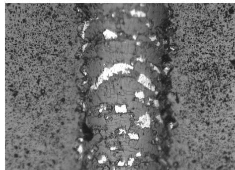
Fig. 9. Scratch failure pictures of the CrN/DLC coating at  $L_{C2}$
