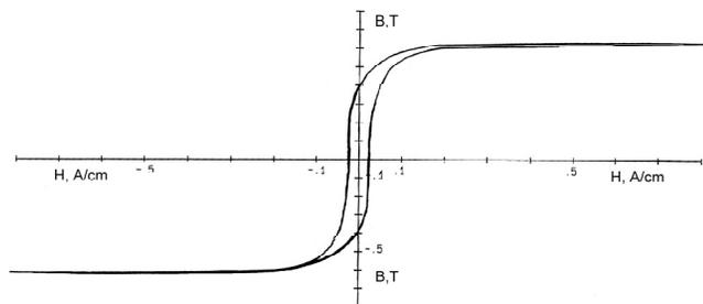
Fig. 4. Hysteresis loop of  $\text{Co}_{69}\text{Mo}_2\text{Fe}_4\text{Si}_{14}\text{B}_{11}$  alloy in as quenched' state
