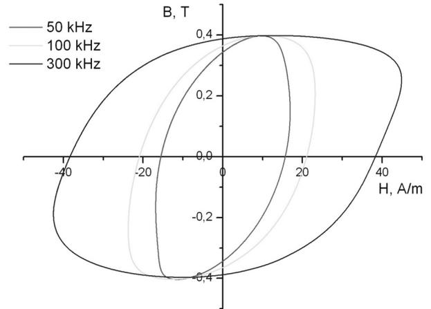
Fig. 9. Hysteresis loops obtained for frequencies in the range of 50-300 kHz for cores from  $Co_{69}Mo_2Fe_4Si_{14}B_{11}$  alloy annealed at 150°C
