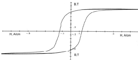
Fig. 8. Hysteresis loops obtained for frequencies 20 kHz for cores from  $Co_{69}Mo_2Fe_4Si_{14}B_{11}$  alloy in 'as quenched' state
