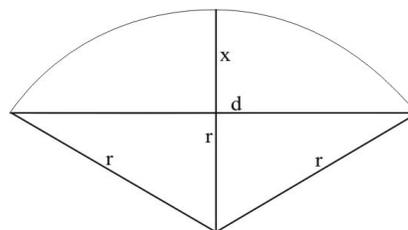
Fig. 3. The method of determining the diameter of a circle, having data:  $d$  - the chord length  $d$  and distance of this chord from the perimeter  $x$
