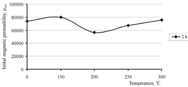
Fig. 6. Influence of annealing temperature on the initial magnetic permeability  $\mu_{start}$  of the studied metallic glass
