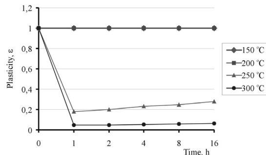
Fig. 10. Dependence of plasticity  $\epsilon$  on annealing time of  $Co_{69}Mo_2Fe_4Si_{14}B_{11}$  metallic glass at various temperature
