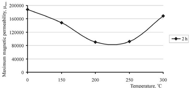
Fig. 7. Influence of annealing temperature on the maximum magnetic permeability  $\mu_{max}$  of the investigated material
