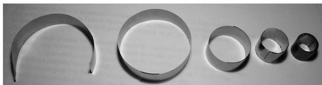
Fig. 2. Exemplary view of relaxed ribbon after losing inner constraints
