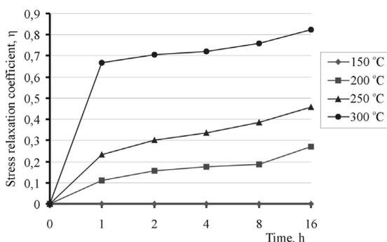
Fig. 11. Dependence of stress relaxation coefficient  $\eta$  on annealing time at different temperatures
