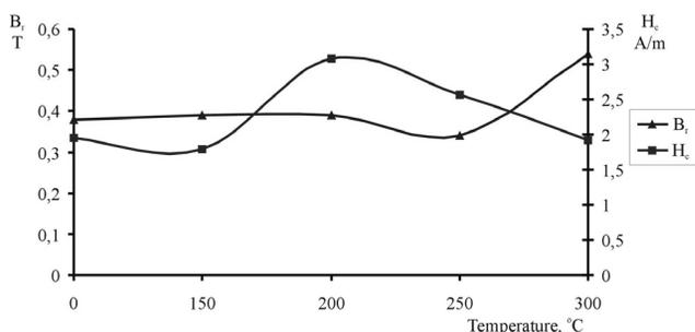
Fig. 5. Influence of annealing temperature on the remanence  $B_r$  and coercive force  $H_c$  of  $\text{Co}_{69}\text{Mo}_2\text{Fe}_4\text{Si}_{14}\text{B}_{11}$  alloy
