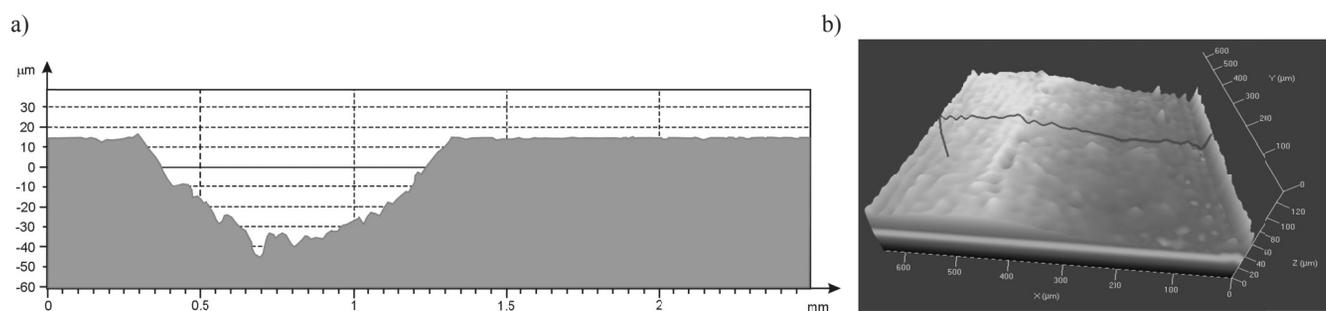
Fig. 13. Shape and depth (a) and half topography (b) of the wear trace after the abrasion wear test of X6Cr13steel with 10% addition of X2CrNiMo25-7-4 steel powder
