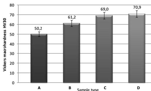
Fig. 9. Vickers macrohardness HV<sub>30</sub> for sintered materials
