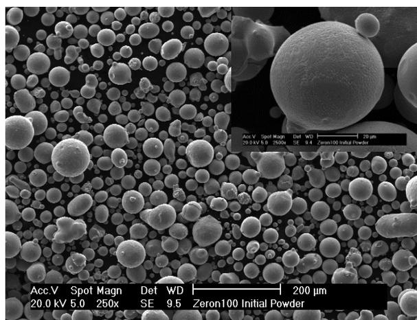
Fig. 2. Morphology of as-atomized super duplex stainless steel X2CrNiMo25-7-4 powder
