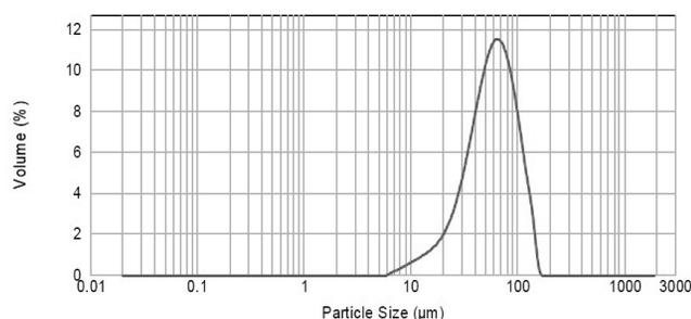
Fig. 8. Particle size distribution of ferritic powder X6Cr13
