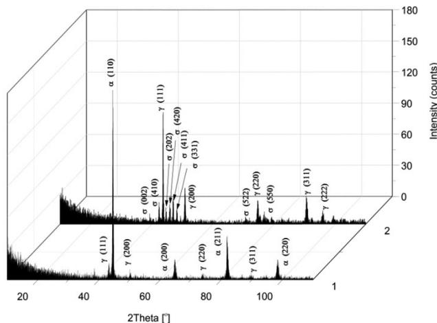
Fig. 5. X-ray diffraction patterns of powder X2CrNiMo25-7-4: 1) initial powder, 2) after heat treatment, 900°C/10 h, precipitation of  $\sigma$ -phase
