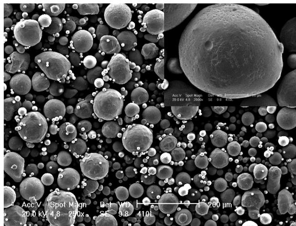
Fig. 1. Morphology of ferritic stainless steel X6Cr13 powder
