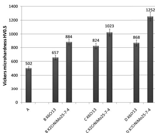
Fig. 10. Vickers microhardness HV<sub>0.5</sub> for different grain in sintered materials
