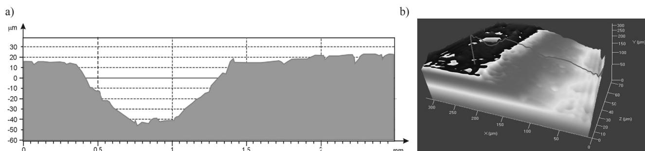
Fig. 12. Shape and depth (a) and half topography (b) of the wear trace after the abrasion wear test of X6Cr13steel with 5% addition of X2CrNiMo25-7-4 steel powder
