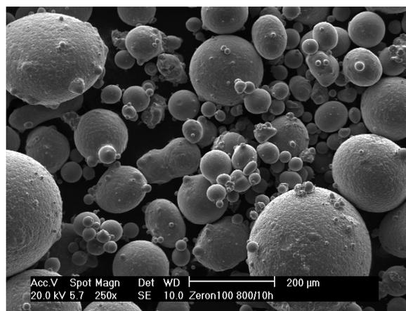
Fig. 3. Morphology of coarse particles of super duplex stainless steel X2CrNiMo25-7-4 after aging at  $900^\circ\text{C}$  for  $10 \text{ h}$ , SEM
