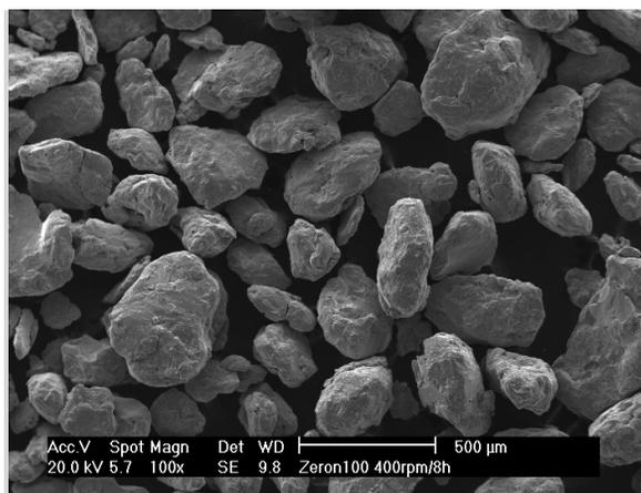
Fig. 4. Morphology of particles of super duplex stainless steel X2CrNiMo25-7-4 after milling
