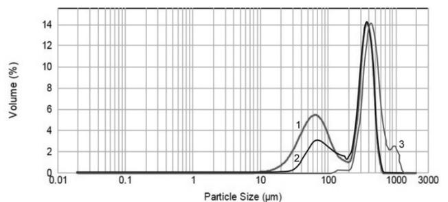
Fig. 7. Particle size distribution of initial powder X2CrNiMo25-7-4 (1), after heat treatment at 900°C/10 h (2), after milling at 400 rpm/8 h (3)
