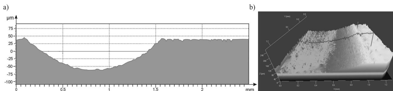
Fig. 11. Shape and depth (a) and half topography (b) of the wear trace after the abrasion wear test of X6Cr13steel
