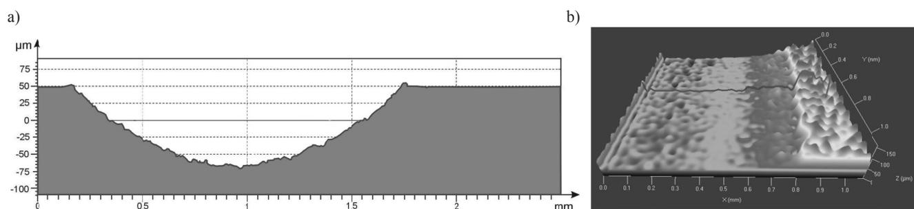
Fig. 14. Shape and depth (a) and half topography (b) of the wear trace after the abrasion wear test of X6Cr13steel with 15% addition of X2CrNiMo25-7-4 steel powder
