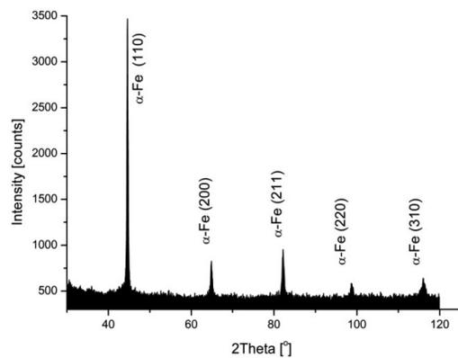
Fig. 6. X-ray diffraction patterns of powder X6Cr13
