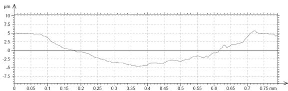
Fig. 16. Wear resistance investigation profile of the 32CrMoV12-28, remelted with 1.2 kW laser power
