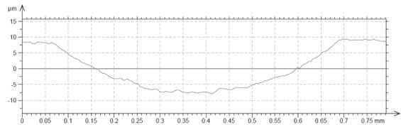
Fig. 13. Wear resistance investigation profile of the X40CrMoV5-1, remelted with 1.6 kW laser power
