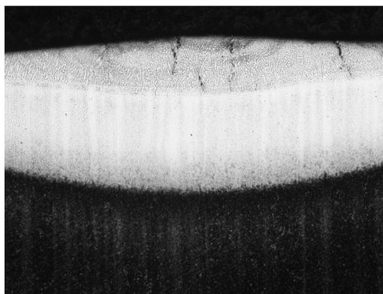
Fig. 4. Shape of cross-section of the laser remelted samples of X40CrMoV5-1 with laser power 2.0 kW, mag. 50x
