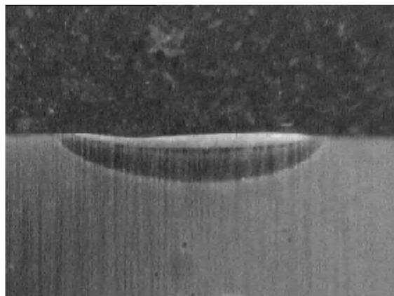
Fig. 3. Shape of cross-section of the laser remelted samples of 32CrMoV12-28 with laser power 2.0 kW, mag. 200x
