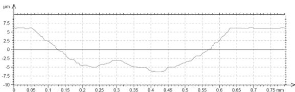
Fig. 18. Wear resistance investigation profile of the 32CrMoV12-28, remelted with 2.0 kW laser power
