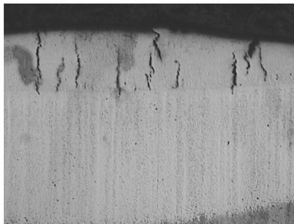
Fig. 10. Structure of the laser remelted samples of 32CrMoV12-28, laser power 2.3, mag. 50x
