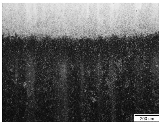
Fig. 5. Structure of the laser remelted samples of X40CrMoV5-1 with laser power 2.0 kW
