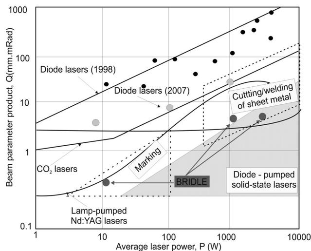
Fig. 1. Parameters of the laser beam for different materials treatment applications [according to: BRIDLE]
