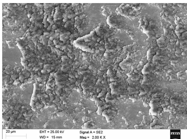
Fig. 7. Surface of the X40CrMoV5-1 sample after wear resistance test, laser power 2.3 kW
