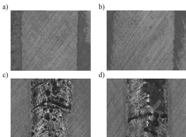
Fig. 2. Shape of the laser tray of the 32CrMoV12-28 steel remelted with BN powder, laser power a) 1.2 kW, b) 1.6 kW, c) 2.0 kW, d) 2.3 kW, mag. 10x
