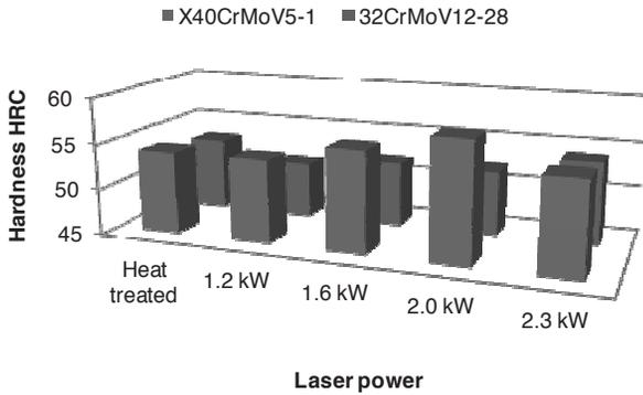
Fig. 11. Hardness measurements results of the remelted surface of X40CrMoV5-1 and 32CrMoV12-28 hot work tool steels
