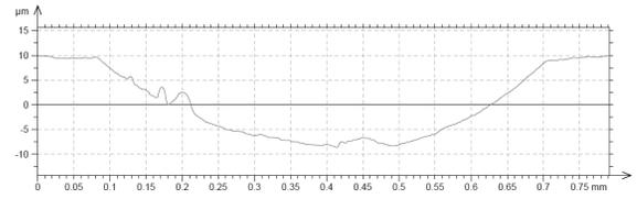
Fig. 14. Wear resistance investigation profile of the X40CrMoV5-1, remelted with 2.0 kW laser power
