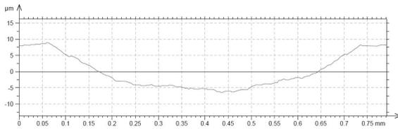
Fig. 12. Wear resistance investigation profile of the X40CrMoV5-1, remelted with 1.2 kW laser power
