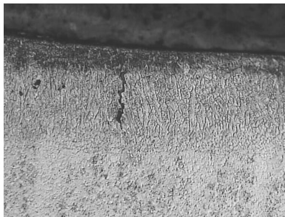
Fig. 9. Structure of the laser remelted samples of 32CrMoV12-28, laser power 2.0 kW, mag.200x
