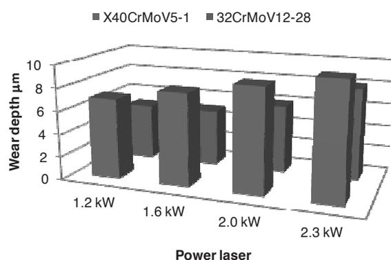
Fig. 20. Maximal wear depth of the remelted surface of X40CrMoV5-1 and 32CrMoV12-28 hot work tool steels
