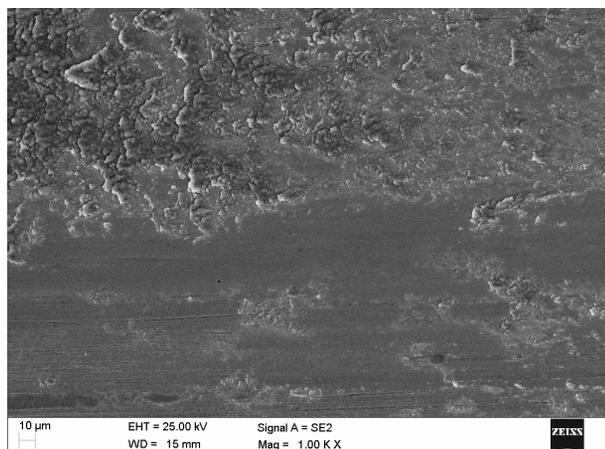
Fig. 8. Surface of the 32CrMoV12-28 -1 sample after wear resistance test, laser power 2.3 kW
