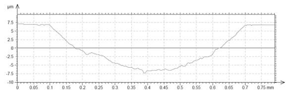
Fig. 19. Wear resistance investigation profile of the 32CrMoV12-28, remelted with 2.3 kW laser power
