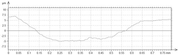
Fig. 17. Wear resistance investigation profile of the 32CrMoV12-28, remelted with 1.6 kW laser power
