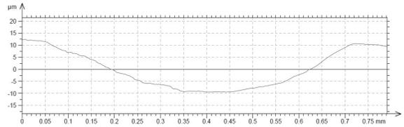
Fig. 15. Wear resistance investigation profile of the X40CrMoV5-1, remelted with 2.3 kW laser power
