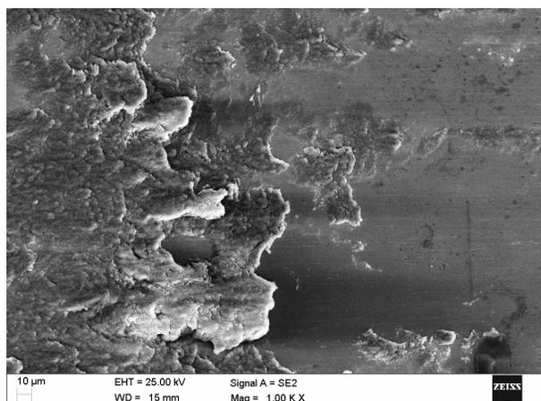
Fig. 6. Surface of the X40CrMoV5-1 sample after wear resistance test, laser power 1.2 kW
