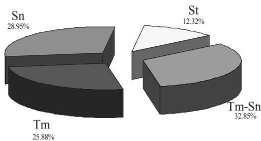
Fig. 15. Contribution of N-CIM processing parameters on flexural strength of PP/MMT 1%; Tm - melt temperature, St - stroke time, Sn - stroke number
