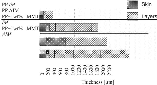
Fig. 13. Thickness of layers for PP and PP+MMT specimens obtained by IM and AIM.
