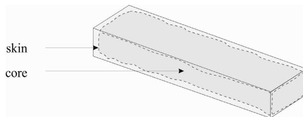
Fig. 5. Schematic illustration of specimen with visible outer (skin) and inner (core) part.
