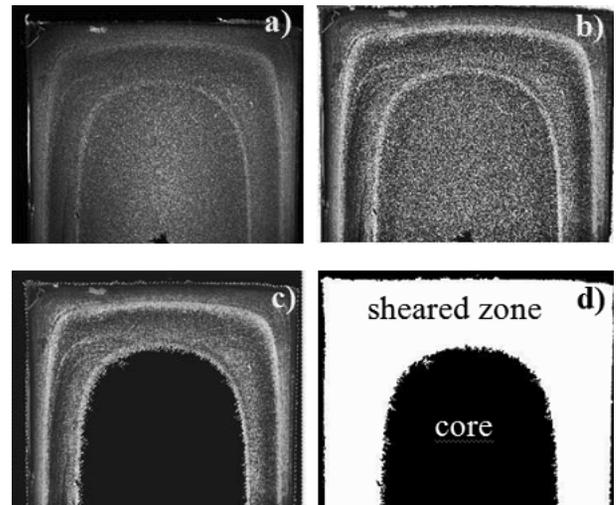
Fig. 11. Order of image analysis of cross sections of investigated specimens; a) direct image from PLM, b) contrast-brightness improvement, c) edge detection, d) mask overlapping
