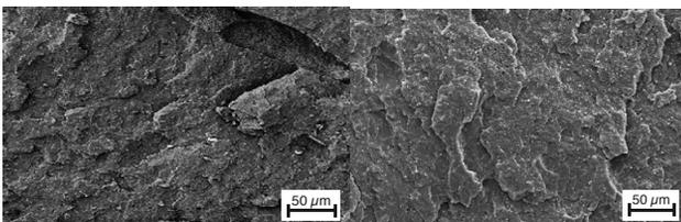
Fig. 9. Cross section of PP specimen with addition of 10wt% of MMT; IM process (left image), AIM process (right image).
