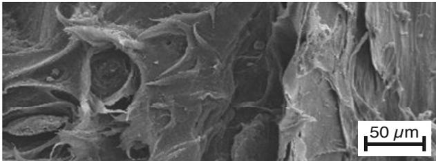
Fig. 8. Cross section of PP specimen; AIM process
