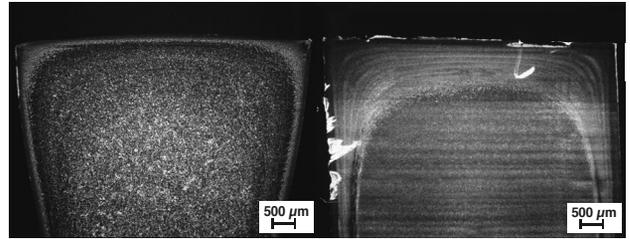
Fig. 10. Cross section of PP specimen with addition; IM process (left image), AIM process (right image).
