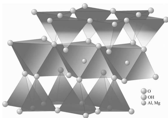
Fig. 4. Schematic illustration of atoms arrangements in a typical MMT layer
