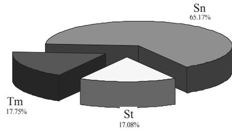
Fig. 16. Contribution of N-CIM processing parameters on flexural strength of PP/MMT 10%; Tm - melt temperature, St - stroke time, Sn - stroke number
