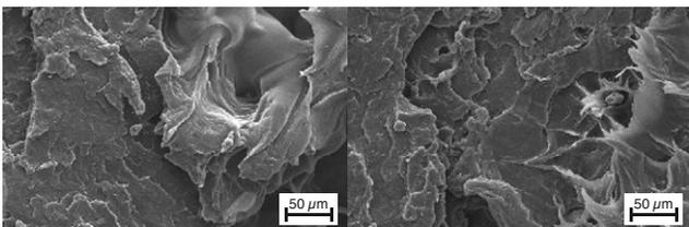
Fig. 9. Cross section of PP specimen with addition of 1wt% of MMT; IM process (left image), AIM process (right image).
