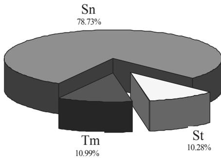
Fig. 14. Contribution of N-CIM processing parameters on flexural strength of PP; Tm - melt temperature, St - stroke time, Sn - stroke number
