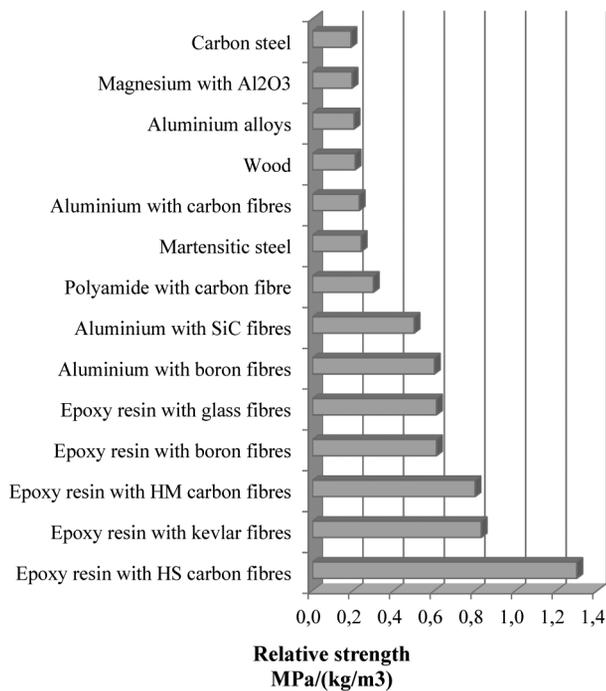
Fig. 1. Comparison of relative strength of selected engineering materials, including composites [19,20]
