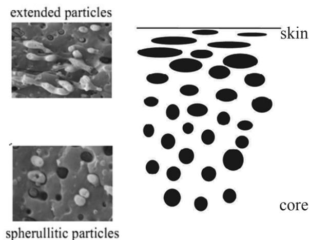
Fig. 6. Shape of particles due to different shearing stress induced during injection molding
