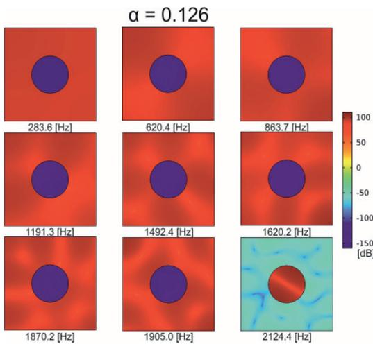
Fig. 3. First nine eigenfrequencies for fill factor  $\alpha=0.126a$
