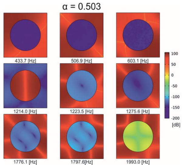
Fig. 7. First nine eigenfrequencies for fill factor  $\alpha=0.503a$
