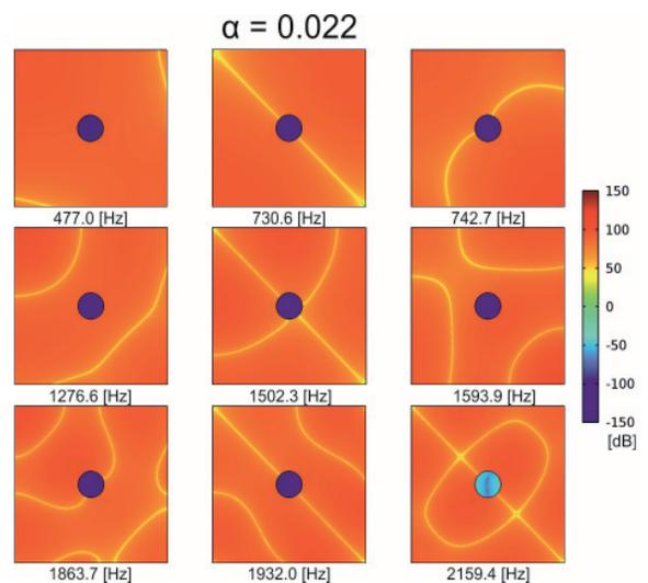
Fig. 2. First nine eigenfrequencies for fill factor  $\alpha=0.022a$
