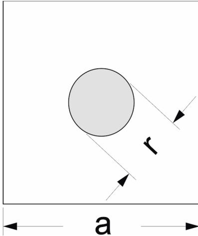
Fig. 1. Phononic crystal primary lattice cell. The rod inside the cell is placed centrally
