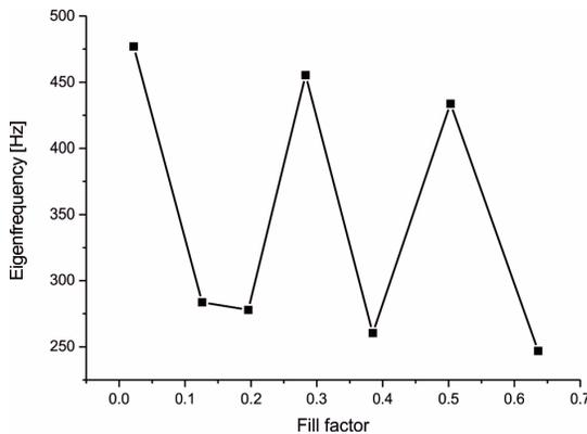
Fig. 9. Fill factor vs. eigenfrequency for first eigenfrequency. The presented lines are only guidelines for the eyes
