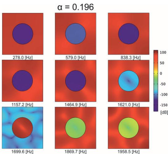
Fig. 4. First nine eigenfrequencies for fill factor  $\alpha=0.196a$
