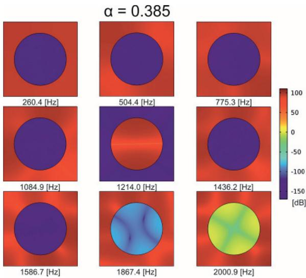
Fig. 6. First nine eigenfrequencies for fill factor  $\alpha=0.385a$
