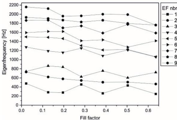
Fig. 10. Fill factor vs. eigenfrequency for first nine eigenfrequencies. The presented lines are only guidelines for the eyes
