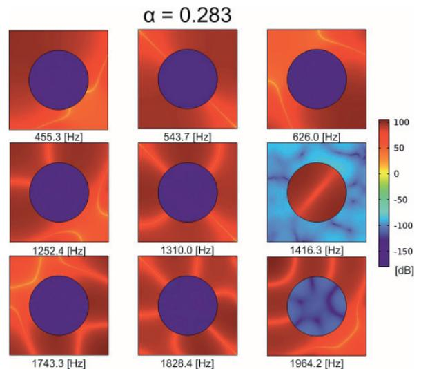
Fig. 5. First nine eigenfrequencies for fill factor  $\alpha=0.283a$
