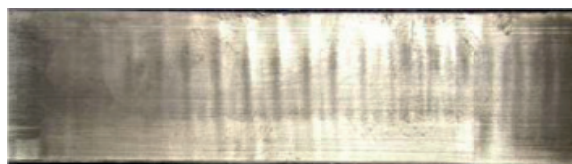
Fig. 3. Sheet steel 11 321 after the DRECE process (rotation 6×180°)
