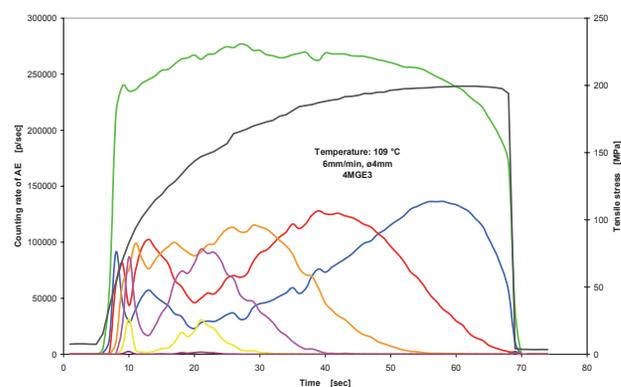
Fig. 3. Record of tensile stress curve with AE – 6 mm/min, 109°C
