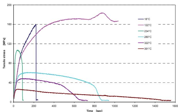
Fig. 12. Comparison of tensile stress curves – 0.6 mm/min
