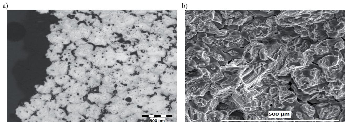
Fig. 15. Testing temperature – 17°C: a) microstructure of sample, b) fracture areas of sample
