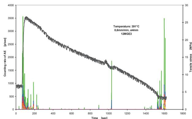
Fig. 11. Record of tensile stress curve with AE – 0.6 mm/min, 391°C
