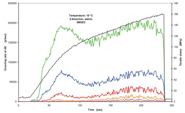
Fig. 8. Record of tensile stress curve with AE – 0.6 mm/min, 18°C
