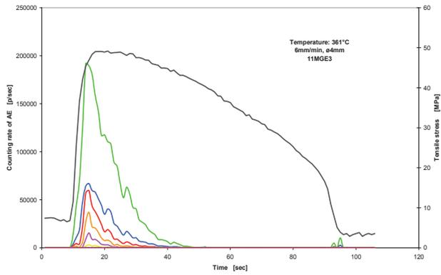
Fig. 6. Record of tensile stress with AE – 6 mm/min, 361°C
