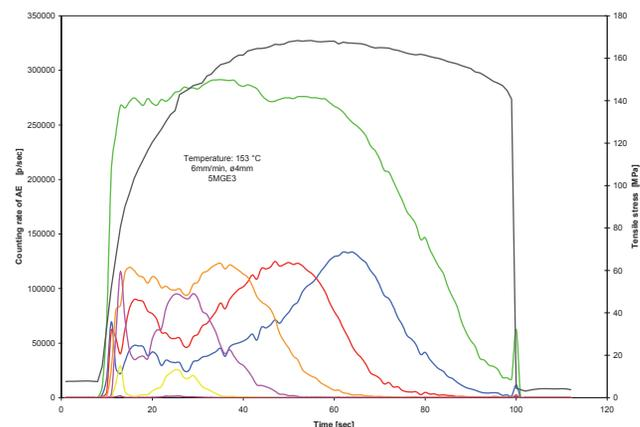
Fig. 4. Record of tensile stress curve with AE – 6 mm/min, 153°C
