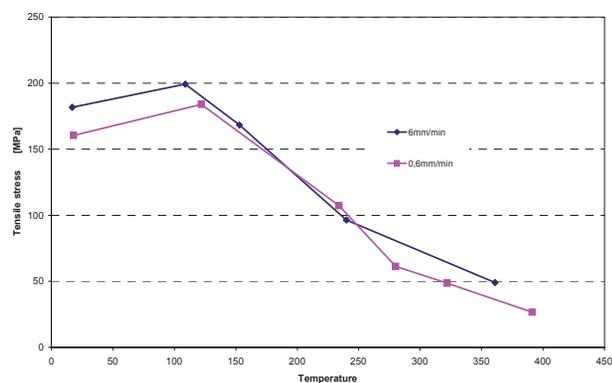
Fig. 13. Comparison of tensile stress curves with crosshead rate 6 and 0.6 mm/min
