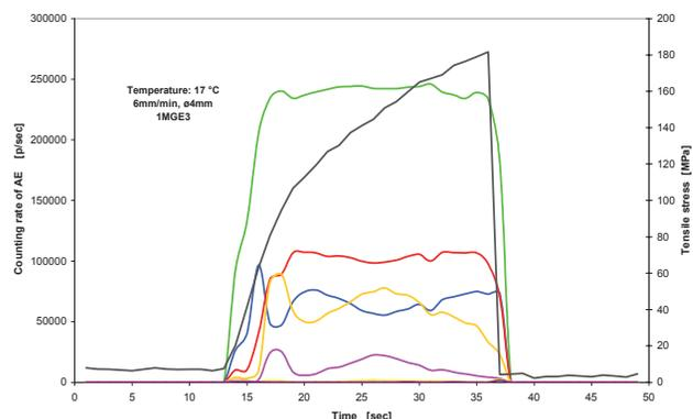
Fig. 2. Record of tensile stress curve with AE – 6 mm/min, 17°C
