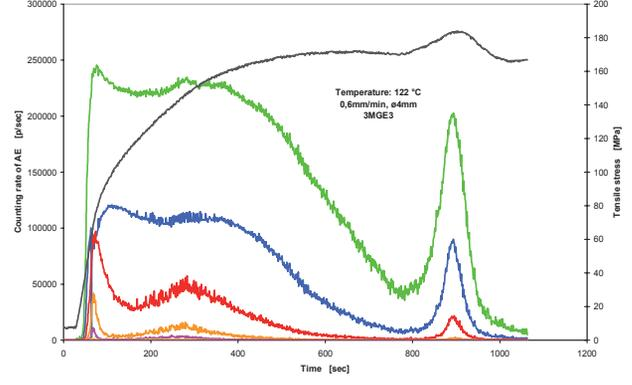
Fig. 9. Record of tensile stress curve with AE – 0.6 mm/min, 122°C
