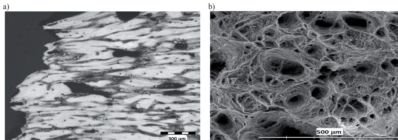
Fig. 18. Testing temperature – 361°C: a) microstructure of sample, b) fracture areas of sample
