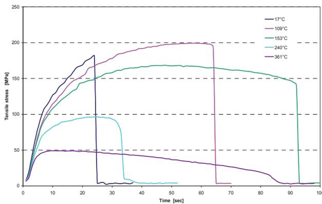
Fig. 7. Comparison of tensile stress curves – 6 mm/min
