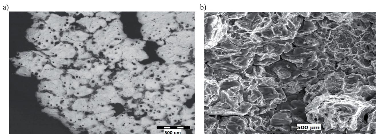
Fig. 17. Testing temperature – 240°C: a) microstructure of sample, b) fracture areas of sample
