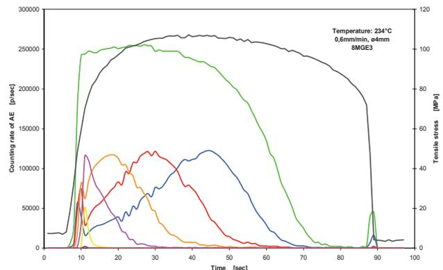
Fig. 10. Record of tensile stress curve with AE – 0.6 mm/min, 234°C
