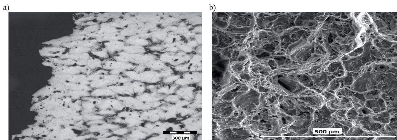
Fig. 16. Testing temperature – 153°C: a) microstructure of sample, b) fracture areas of sample
