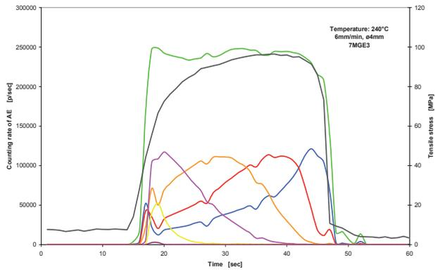
Fig. 5. Record of tensile stress curve with AE – 6 mm/min, 240°C
