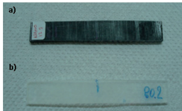
Fig. 4. The samples of: a) nanocomposite reinforced with MWCNT b) polymer material
