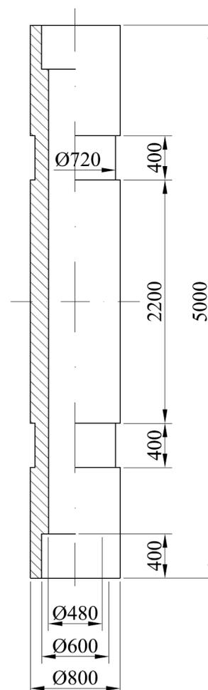
Fig. 2. Geometry of the pipe mould
