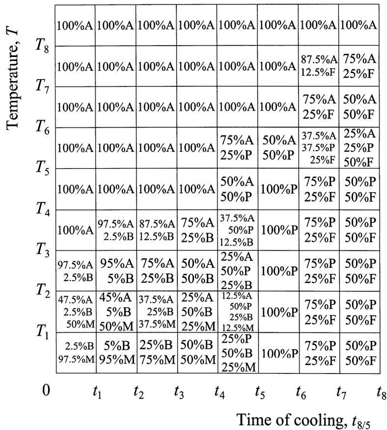
Fig. 1. Contents of ferrite, pearlite, bainite, martensite and austenite at some temperature
