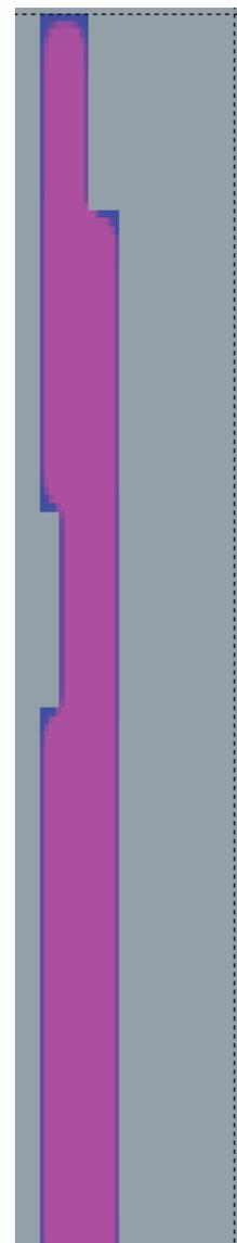
Fig. 5. Distribution of pearlite in quenched pipe mould
