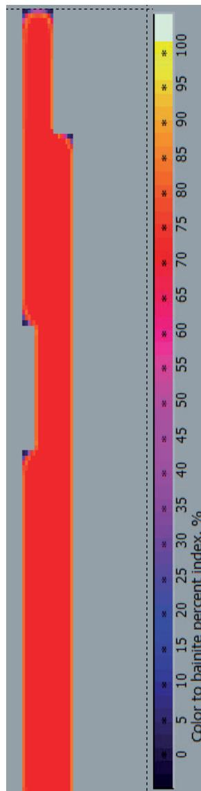
Fig. 4. Distribution of bainite in quenched pipe mould
