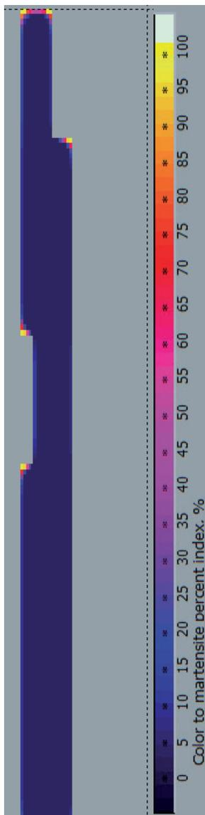
Fig. 3. Distribution of martensite in quenched pipe mould
