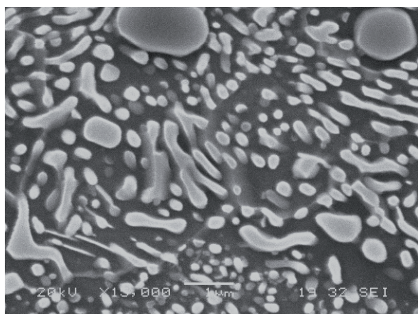
Fig. 7. Microstructure of sample 4, 267 HV10. partially spheroidised and fragmented pearlitic lamellae
