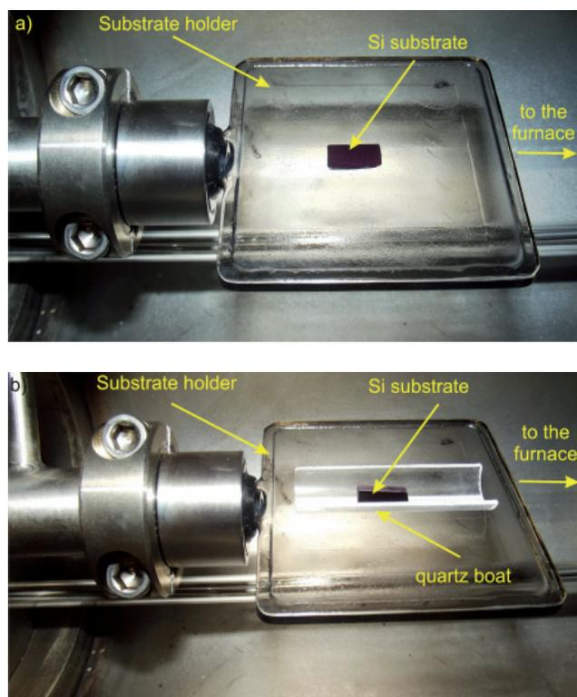
Fig. 2. Two options of placement of specimens in the oven: a) a specimen placed directly on a feeder, b) a specimen placed on a feeder additionally in a quartz boat
