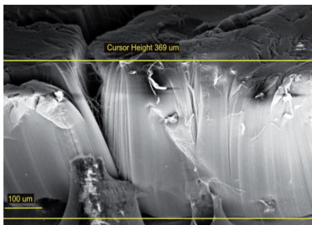
Fig. 11. SEM image of vertically aligned carbon nanotubes synthesised in a quartz boat; mag. 350x
