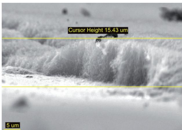
Fig. 7. SEM image of vertically aligned carbon nanotubes; synthesis time 15 min; mag. 4300x
