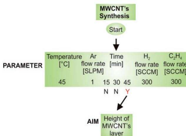
Fig. 1. Diagram showing a graphical concept of selection of carbon nanotubes' synthesis parameters for ensuring a maximum height of their layers
