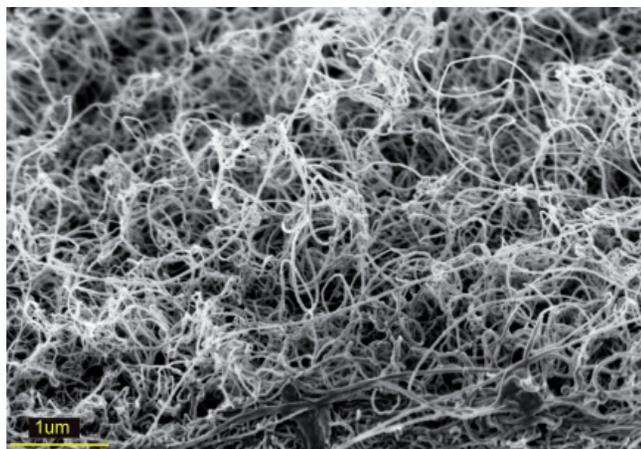
Fig. 3. SEM image of randomly arranged carbon nanotubes; mag. 50 000x
