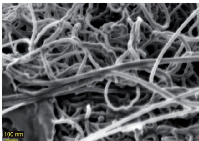
Fig. 5. SEM image of randomly arranged carbon nanotubes; mag. 200 000x
