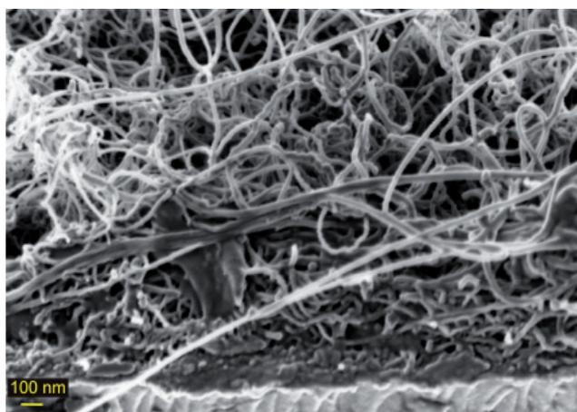
Fig. 4. SEM image of randomly arranged carbon nanotubes; mag. 100 000x
