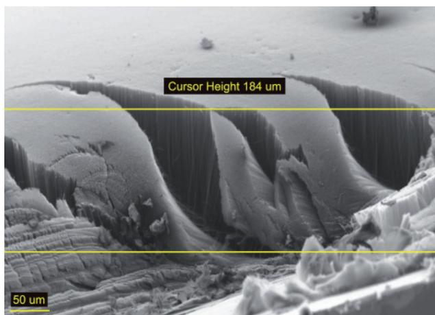
Fig. 10. SEM image of vertically aligned carbon nanotubes; side view (after rotating a specimen by 90°); mag. 285x
