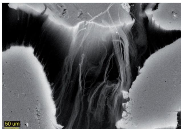
Fig. 9. SEM image of vertically aligned carbon nanotubes; synthesis time 45 min; top view; mag. 500x
