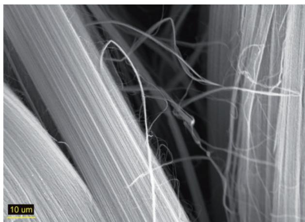
Fig. 12. SEM image of vertically aligned carbon nanotubes synthesised in a quartz boat; mag. 3000x
