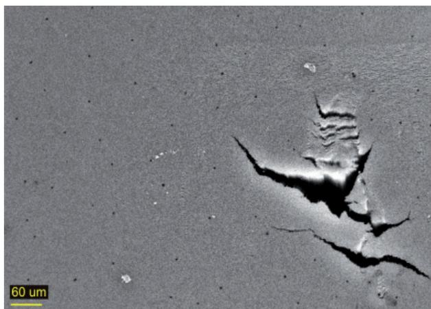
Fig. 8. SEM image of vertically aligned carbon nanotubes; synthesis time 45 min; top view; mag. 400x
