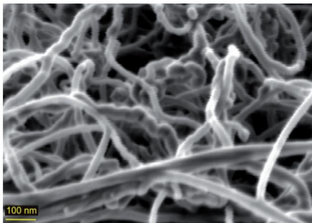
Fig. 6. SEM image of randomly arranged carbon nanotubes; mag. 300 000x
