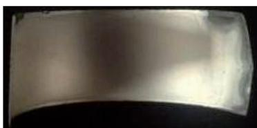
Fig. 16. Fragment of SF12050 superconducting tape, subjected to annealing at 800°C during time of 2 h, view from the side of the silver layer, air cooling
