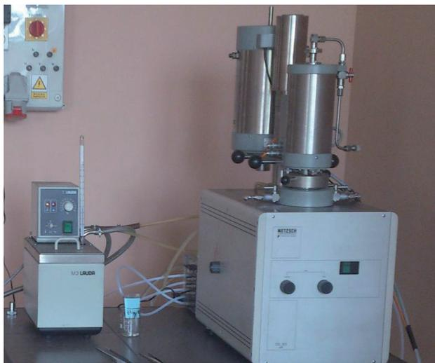
Fig. 2. Differential Scanning Calorimeter NETZSCH STA 409C
