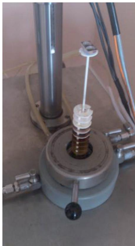
Fig. 3. The interior chamber of the differential scanning calorimeter NETZSCH STA 409C
