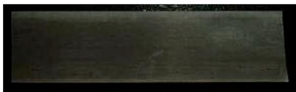
Fig. 9. Fragment of SF12050 superconducting tape, subjected to annealing at 550°C during time of 48 h, view from the side of the substrate, air cooling
