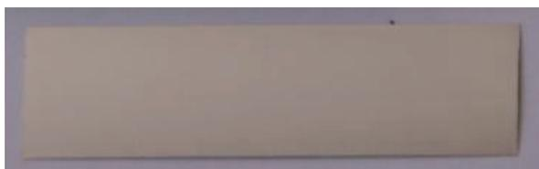
Fig. 7. Fragment of SF12050 superconducting tape, subjected to annealing at 500°C during time of 6 h, view from the side of the silver layer, air cooling
