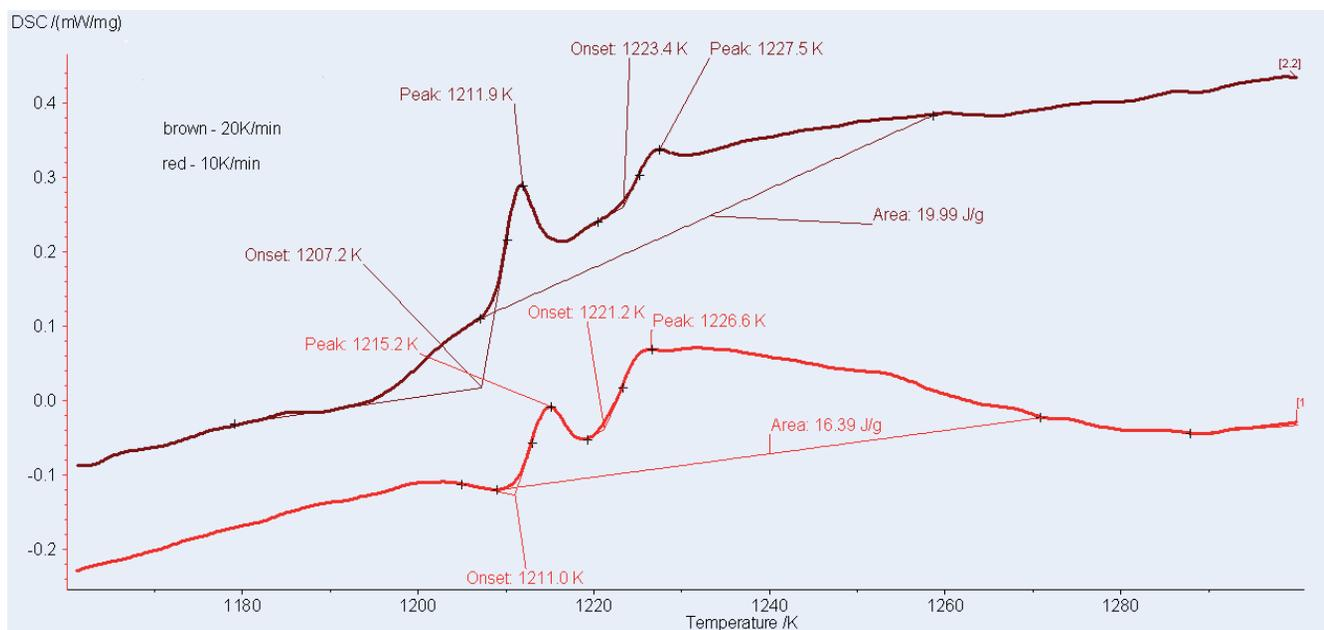
Fig. 5. Clipping the DSC curve in the temperature range 1160 K-1300 K obtained by heating SF12050 tape
