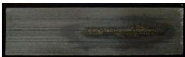
Fig. 15. Fragment of SF12050 superconducting tape, subjected to annealing at 720°C during time of 48 h, view from the side of the substrate, air cooling
