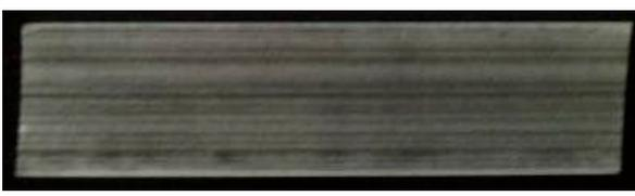
Fig. 11. Fragment of SF12050 superconducting tape, subjected to annealing at 650°C during time of 48 h, view from the side of the substrate, air cooling
