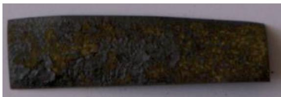
Fig. 18. Fragment of SF12050 superconducting tape, subjected to annealing at 800°C during time of 6 h, view from the side of the substrate, air cooling
