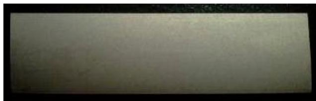
Fig. 6. Fragment of SF12050 superconducting tape, subjected to annealing at 450°C during time of 48 h, view from the side of the silver layer, air cooling
