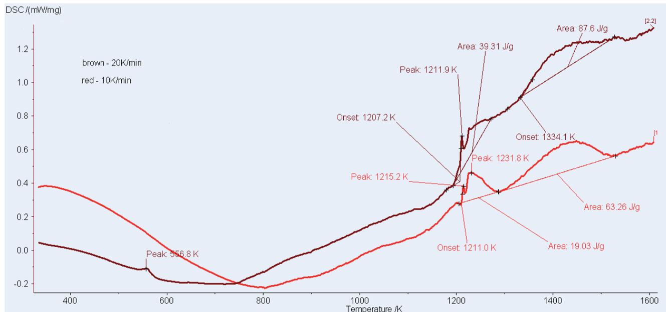
Fig. 4. Segments of DSC curves in the temperature range 300 K-1600 K obtained by heating tape SF12050
