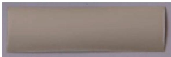
Fig. 12. Fragment of SF12050 superconducting tape, subjected to annealing at 700°C during time of 6 h, view from the side of the silver layer, air cooling
