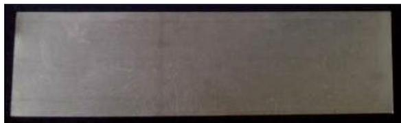
Fig. 8. Fragment of SF12050 superconducting tape, subjected to annealing at 550°C during time of 48 h, view from the side of the silver layer, air cooling
