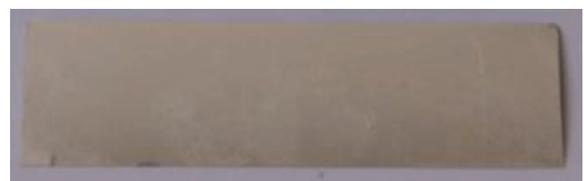
Fig. 10. Fragment of SF12050 superconducting tape, subjected to annealing at 600°C during time of 2 h, view from the side of the silver layer, air cooling
