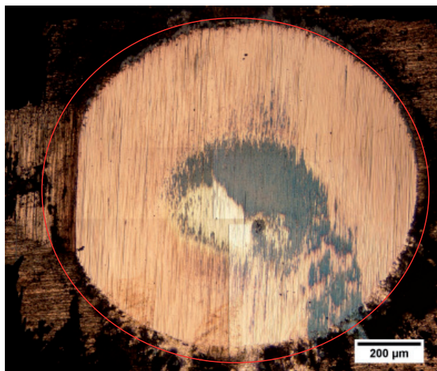
Fig. 14. A wipe made on the surface of the high temperature \text{YBa}_2\text{Cu}_3\text{O}_{7-x} – YBCO 2G HTS superconducting tape coated with Cu, after 2 hours
