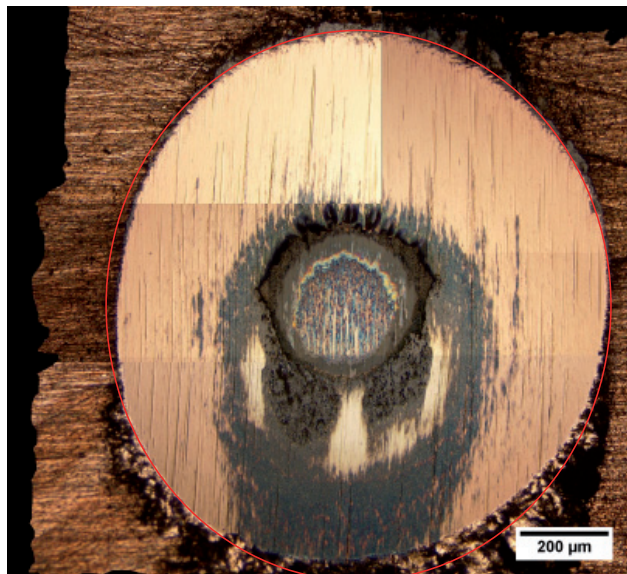
Fig. 15. A wipe made on the surface of the \text{YBa}_2\text{Cu}_3\text{O}_{7-x} – YBCO 2G HTS high temperature superconducting tape coated with Cu, after 3 hours
