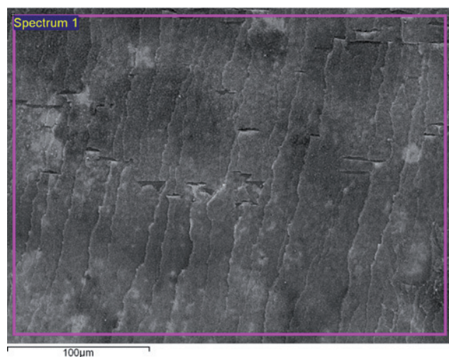
Fig. 11. Randomly selected area in which measurement of the chemical composition distribution layer for superconducting tapes \text{YBa}_2\text{Cu}_3\text{O}_{7-x} – YBCO 2G HTS coated with Cu was carried out
