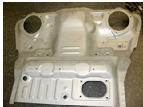
Fig. 9. Complicated sheet metal part produced by sheet hydroforming
