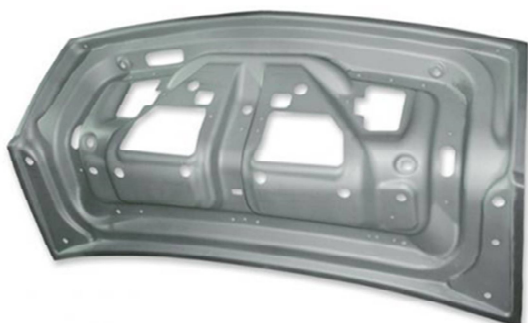
Fig. 3. Trunk-lid panel made of magnesium alloy [8]
