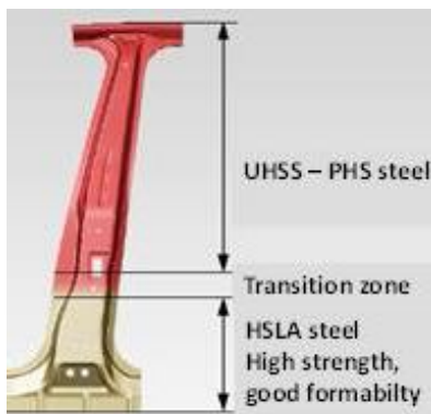
Fig. 13. Hot press forming of a B-pillar applying the so-called Hot Tailor Welded (HTW) concept
