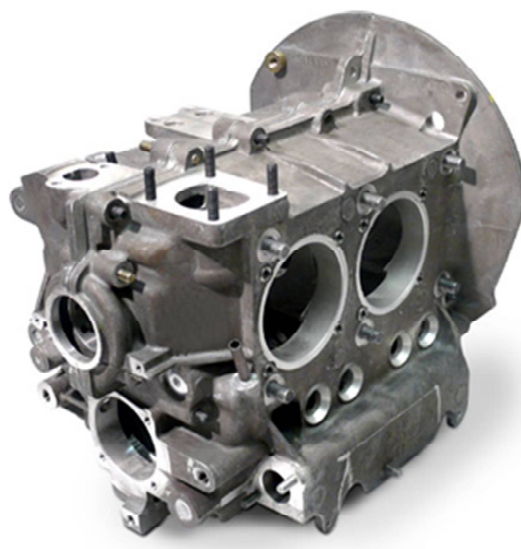
Fig. 5. Automotive engine block made of magnesium alloy
