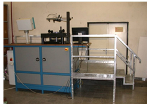
Fig. 14. Complex formability testing machine equipped with Vialux optical strain measurement system
