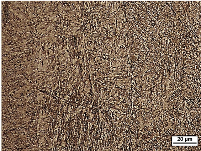
Fig. 13. Microscopic image of the S960Q steel welded with the Union X90 filler of sample 8
