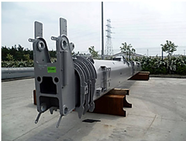
Fig. 3. View of a finished telescopic boom of a self-propelled crane [7]
