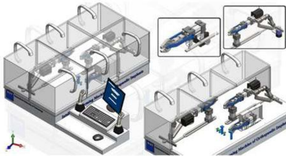
Fig. 9. Conceptual design of a CNC machine which uses hydraulics as driver
