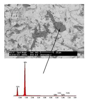
Fig. 3. Scanning electron micrograph of samples treated with shot-peening. Microanalysis of inclusion detected on the surface that corresponds with  $Al_2O_3$
