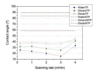
Fig. 7. Variation of contact angle with scanning rate
