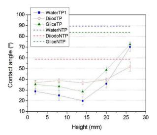
Fig. 8. Variation of contact angle with plasma torch height
