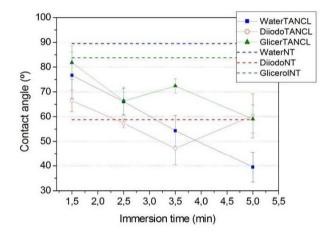
Fig. 4. Evolution of contact angle with immersion time of acid etched samples
