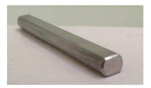
Fig. 1. Specimen of SAF 2205 stainless steel for surface treatments.
