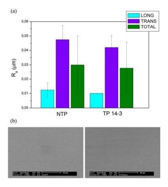
Fig. 9. (a) Surface roughness in both longitudinal and transversal directions of the test treated (TP 14-3) and untreated (NTP) specimens. (b) SEM images of treated and untreated samples
