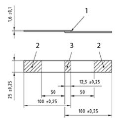
Fig. 2. Scheme of the shear test specimens (1: adhesive line; 2: grip area; 3: overlap area). Dimensions are given in mm.
