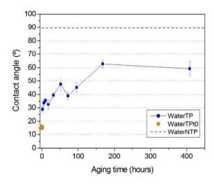
Fig. 10. Evolution of contact angle with aging time after APPJ
