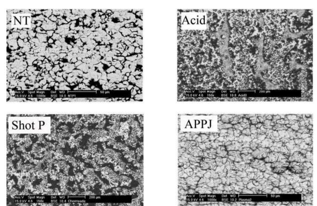
Fig. 11. (a) Shear strength and (b) micrographs of rupture failure of treated and untreated samples
