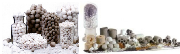
Fig. 3. Different forms of porous solid materials (sorbents, catalysts): spherical pellets; cylindrical pellets; tablets, tubes
