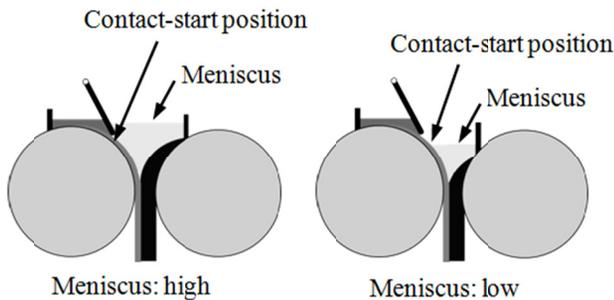
Fig. 16. Schematic illustration showing the relationship between the position of the meniscus and the contact-start position
