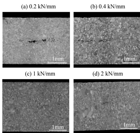
Fig. 8. Cross section of as-cast 5182 strip cast at 60 m/min
