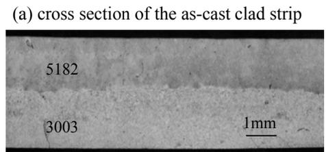
(a) cross section of the as-cast clad strip
