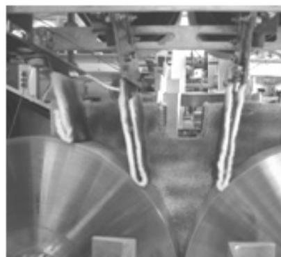
Fig. 6. Photograph of the vertical type twin roll caster equipped with a scraper
