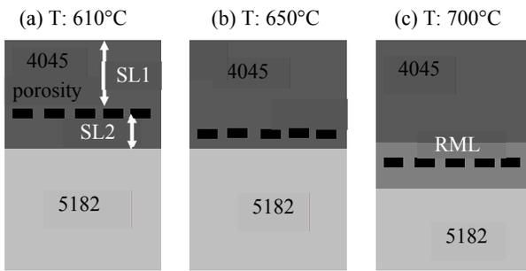
Fig. 12. schematic illustration of porosity occurred at the three layers clad strip shown in Fig. 11. T: poring temperature of 4045 molten metal, SL1: solidified layer by the lower roll, SL2: solidified layer by 5182 strip, RML: re-melted and reacted layer
