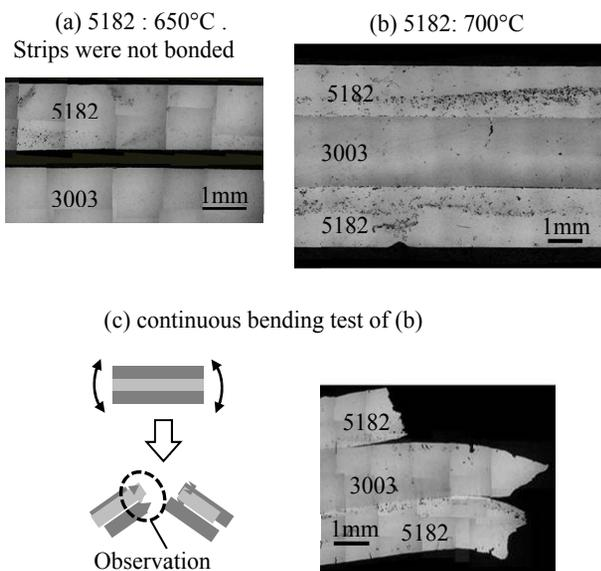
Fig. 9. Cross section of as-cast type A1 three layers clad strip consisting of the 3003 base strip and 5182 overlay strip, and result of continuous bending test
