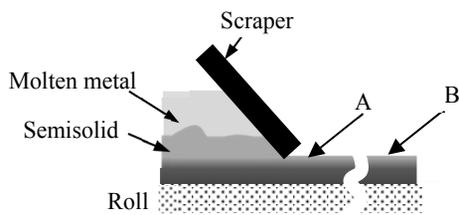
Fig. 15. Schematic illustration showing the temperature of the scribed surface. Temperature at position B is lower than position A
