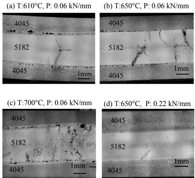
Fig. 11. Cross section of as-cast three layers clad strip consisting of the 5182 base strip and 4045 overlay strip. Pouring temperature of the 5182 base strip was 650°C. Roll load of the lower twin roll caster was 0.22 kN/mm. T: pouring temperature of the 4045 overlay strip, P: roll load of the upper twin roll caster to cast the base strip
