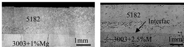
Fig. 10. Cross section of as-cast three layers clad strip consisting of the 5182 overlay strip and the modified 3003 base strip. Pouring temperature of the 5182 overlay strip was 650°C
