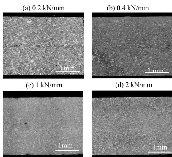
Fig. 7. Cross section of as-cast 5182 strip cast at 30 m/min
