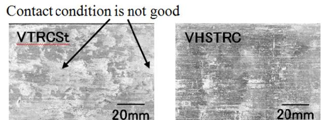
Fig. 2. Surfaces of as-cast 5182 strips cast at 90 m/min by a vertical type twin roll caster for steel and a vertical type high speed twin roll caster for aluminium alloy
