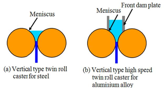
Fig. 1. Schematic illustration of a vertical type twin roll caster for steel and a vertical type high speed twin roll caster for aluminium alloy
