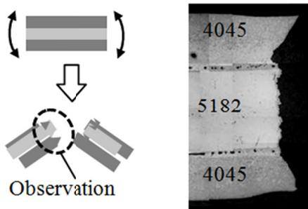
Fig. 13. Result of the continuous bending test of the three layers clad strip consisting of 5182 base strip and 4045 overlay strip
