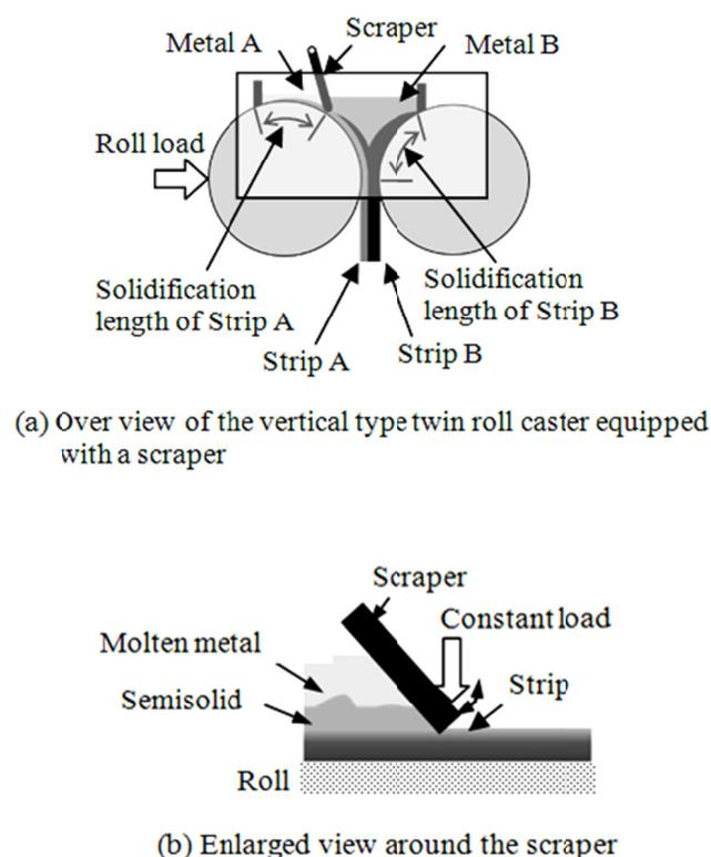
Fig. 5. Schematic illustration of the vertical type twin roll caster equipped with a scraper and enlarged view around the scraper
