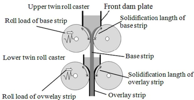
Fig. 3. Schematic illustration of the vertical type tandem twin roll caster
