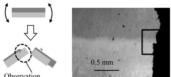
(b) result of the continuous bending test of the as-cast clad strip
