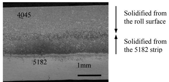
Fig. 17. Cross section of two layers clad strip consisting of the 5182 strip and 4045 strip
