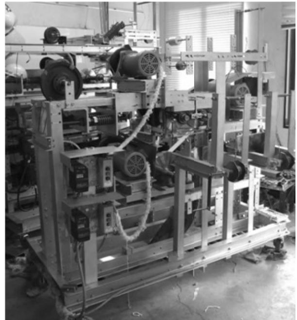
Fig. 4. Photograph of the vertical type tandem twin roll caster
