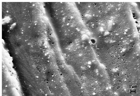
Fig. 19. The structure of the turn of the composite polymeric material having a share of 3% of Cu nanowires, scanning electron microscope
