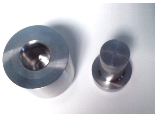
Fig. 1. Steel mold with an inner diameter of 30 mm
