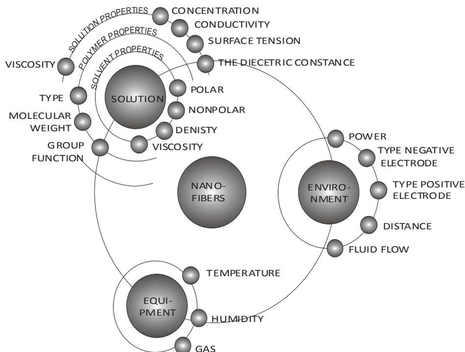
Fig. 26. Graphical presentation of process conditions, environmental conditions and properties of solution influencing the diameter of fibers obtained
