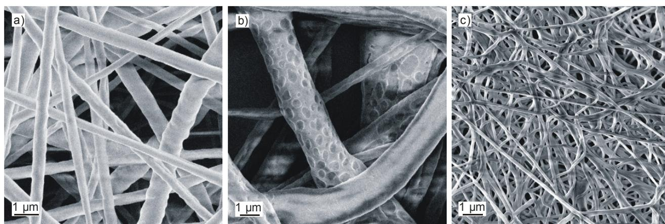
Fig. 9. Comparison of influence of solvents' properties on the structure of the obtained PCL fibers from the following solutions; a) mixture of formic acid and hydrochloric acid at a rate of 70:30; b) mixture of tetrahydrofuran and dimethyl sulfoxide at a rate of 70:30, c) mixture of chloroform and methanol at a rate of 70:30
