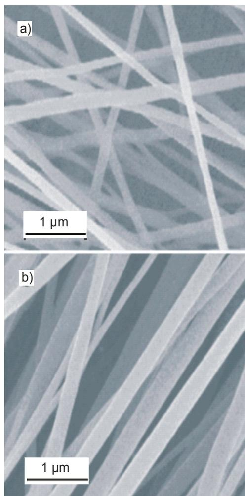
Fig. 10. Influence of rotational speed of collector on spatial arrangement of fibers deposited with the rotation speed: a) 200 rev./min, b) 1400 rev./min
