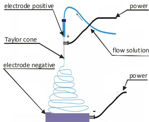
Fig. 3. Nanofibers electrospinning schematic
