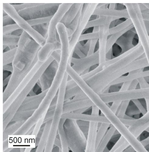
Fig. 13. Geometrical characteristics of double-component fibers obtained by dissolving PCL granulate with the molecular mass of  $M_w = 70,000-90,000$  g/mol using 10% mixture of hydrochloric acid and formic acid with mass ratio of 70:30 with AlphaSan addition with fraction of 5%; SEM
