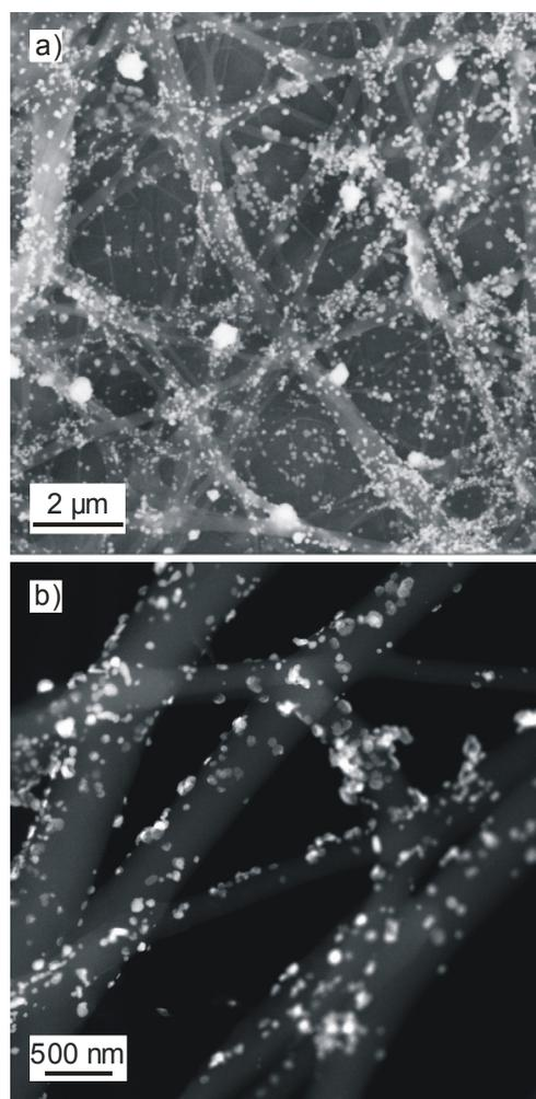
Fig. 11. Geometrical characteristics of double-component fibers obtained by dissolving PCL granulate using 10% mixture of hydrochloric acid and formic acid with mass ratio of 70:30 with addition of  $\text{AgNO}_3$ : a) 3%, b) 25%; photographs taken after precipitation of silver in 2% ascorbic acid solution; a) SEM, b) TEM (HAADF)
