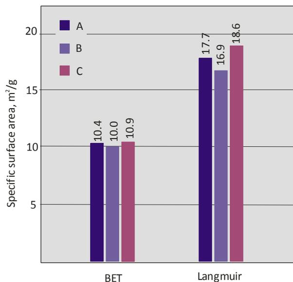
Fig. 17. BET and Langmuir specific surface area of PCL fibers with the molecular mass of  $M_w = 70,000$ – $90,000$  g/mol obtained from 10% mixture of formic acid and hydrochloric acid with mass ratio of 70:30 with addition of AlphaSan with fraction of: A) 1%, B) 3%, C) 5%
