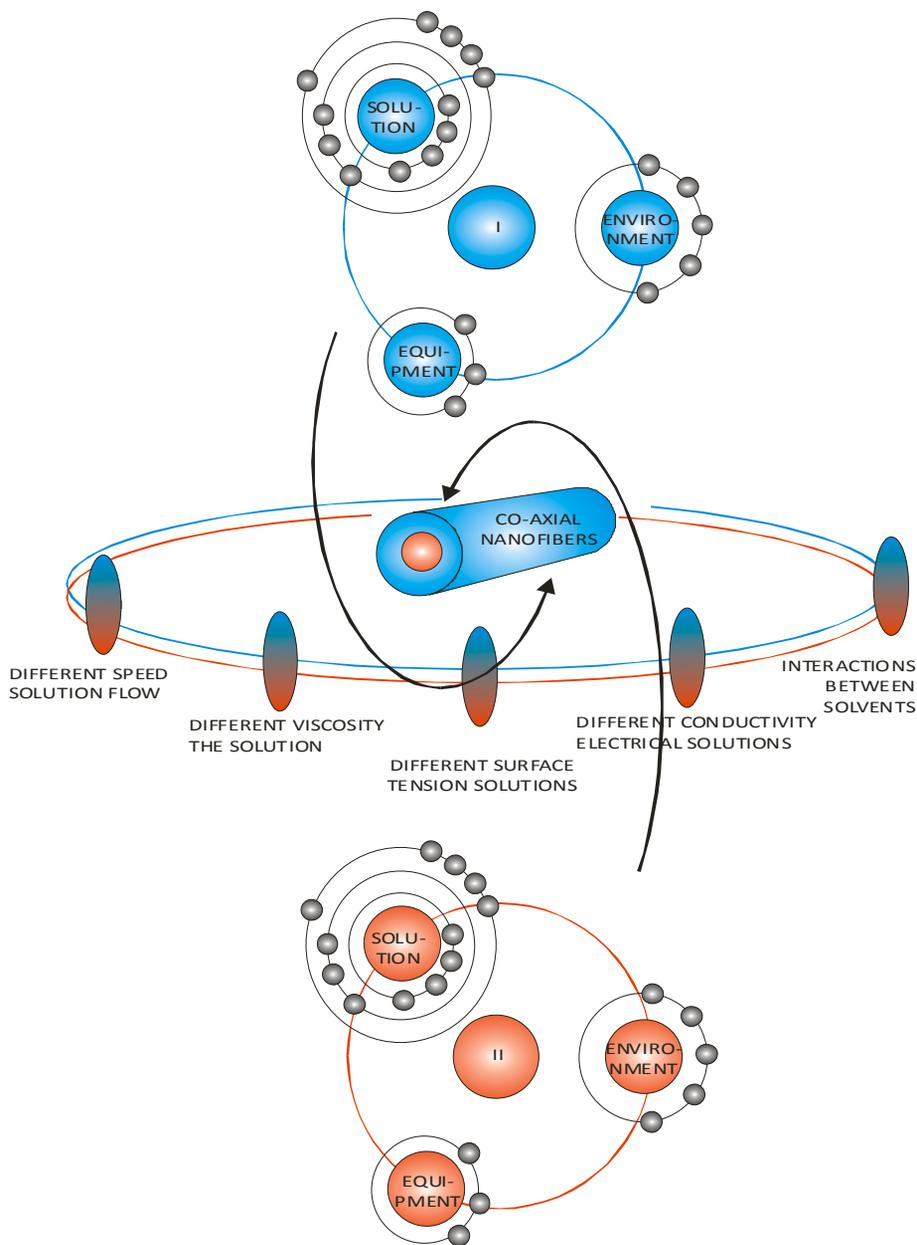
Fig. 27. Conditions underlying the creation of core-shell nanofibers: conditions influencing the core solution are shown in blue, conditions influencing the external shell solution are shown in orange, differences and interactions between solutions are shown in orange; own study
