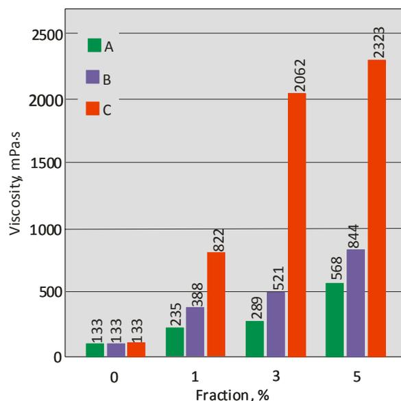
Fig. 6. Change of dynamic viscosity of polycaprolactone solutions ( $M_w = 70,000-90,000 \text{ g/mol}^1$ ) with the fraction of 9.5-10%, obtained by dissolving PCL granulate in the mixture of formic acid and hydrochloric acid (mass ratio of 70:30) and by adding 0-5% of  $\text{AgNO}_3$  (A), AlphaSan (B), chitosan (C)
