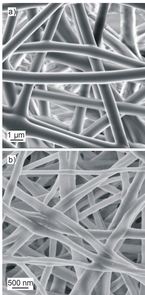
Fig. 21. Geometrical characteristics of core-shell composite obtained from: a) 12% solution of polyvinyl alcohol in the coating at a flow rate of 1 ml/h and the natural oil in the core at a flow rate of 0.1 ml/h; b) 10% solution of polycaprolactone with 3% additive of silver in the coating at a flow rate of 1.0 ml/h and 10% solution of polycaprolactone with 2.5% additive of chitosan and 2.5% additive of hyaluronic acid and gold in the core at a flow rate of 0.1 ml/h; SEM
