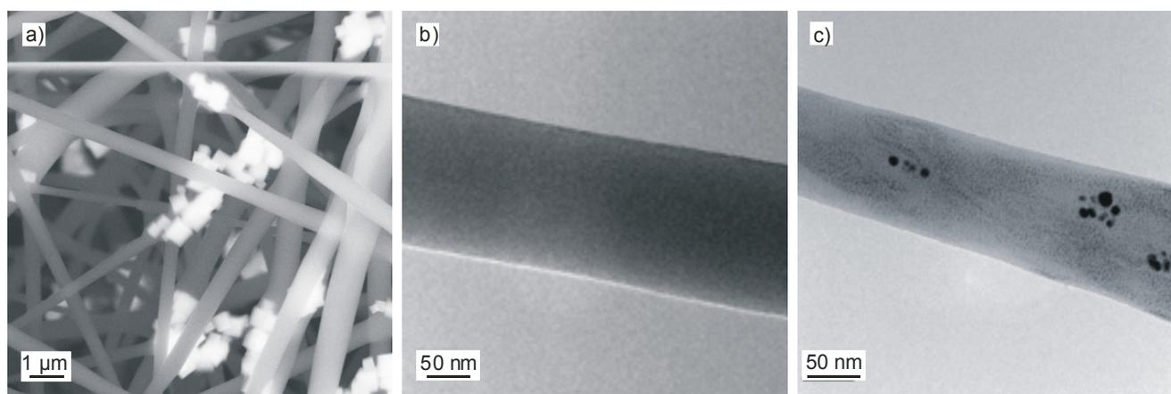
Fig. 15. Geometrical characteristics of double-component fibers obtained by dissolving PCL granulate with the molecular mass of  $M_w = 70,000-90,000$  g/mol using 10% mixture of hydrochloric acid and formic acid with mass ratio of 70:30 with addition of: a) 5% of AlphaSan b) 1% of chitosan, c) 1%  $\text{AgNO}_3$ , after precipitation of silver in 2% ascorbic acid solution; photographs with: a) SEM; b) and c) TEM
