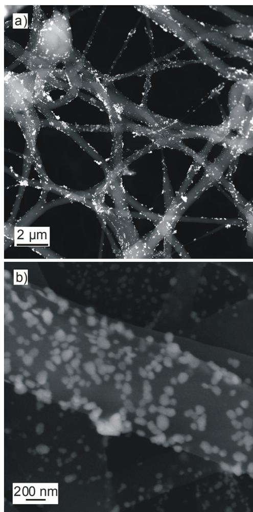
Fig. 12. Geometrical characteristics of double-component fibers obtained by dissolving PCL granulate with the molecular mass of  $M_w = 70,000-90,000$  g/mol using 10% mixture of hydrochloric acid and formic acid with mass ratio of 70:30 with addition of 25% of  $AgNO_3$ ; photographs taken after precipitation of silver in 2% ascorbic acid solution; a) TEM (HAADF), c) SEM
