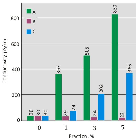
Fig. 8. Change of electric conductivity of polycaprolactone solutions ( $M_w = 70,000-90,000$  g/mol) with the fraction of 9.5-10%, obtained by dissolving PCL granulate in the mixture of formic acid and hydrochloric acid (mass ratio of 70:30) and by adding 0-5% of  $\text{AgNO}_3$  (A), AlphaSan (B), chitosan (C)
