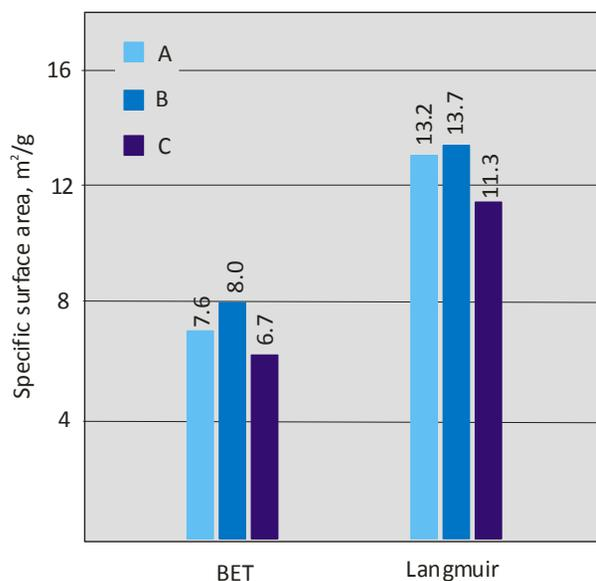
Fig. 18. BET and Langmuir specific surface area of PCL fibers with the molecular mass of  $M_w = 70,000$ – $90,000$  g/mol obtained from 10% mixture of formic acid and hydrochloric acid with mass ratio of 70:30 with addition of chitosan with fraction of: A) 1%, B) 3%, C) 5%
