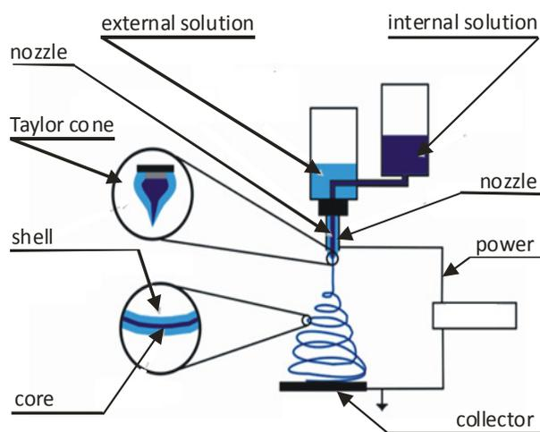
Fig. 4. Simplified co-axial electrospinning
