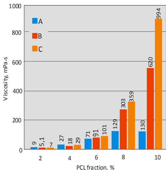
Fig. 5. Change of viscosity of polycaprolactone solution with fraction of 2-10% dissolved in mixture of hydrochloric acid and formic acid (A), chloroform and methanol (B) and a mixture of tetrahydrofuran and dimethyl sulfoxide (C)
