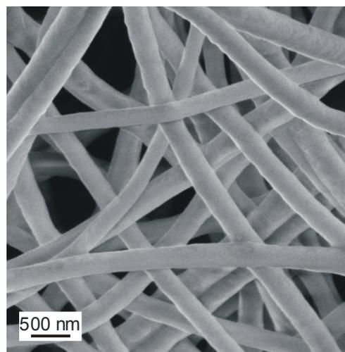
Fig. 20. Geometrical characteristics of core-shell composite obtained of 10% solution of polycaprolactone from which a core and a coating of fibers were obtained, the flow rate of 0.1 ml/h in the shell and the core; SEM
