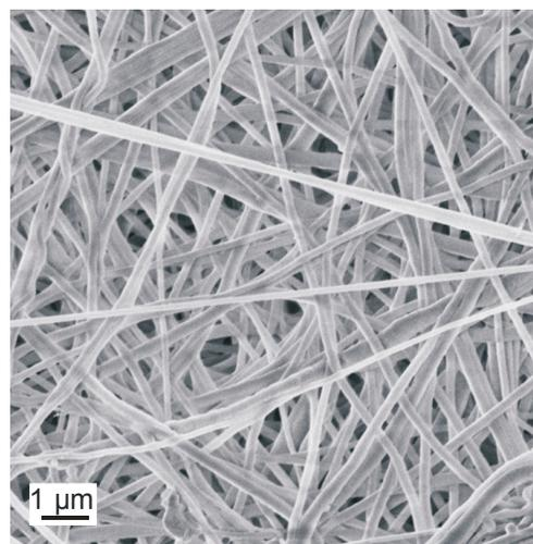
Fig. 14. Geometrical characteristics of double-component fibers obtained by dissolving PCL granulate with the molecular mass of  $M_w = 70,000-90,000$  g/mol using 10% mixture of hydrochloric acid and formic acid with mass ratio of 70:30 with addition of chitosan with fraction of 5%; photographs taken with SEM technique in InLens mode
