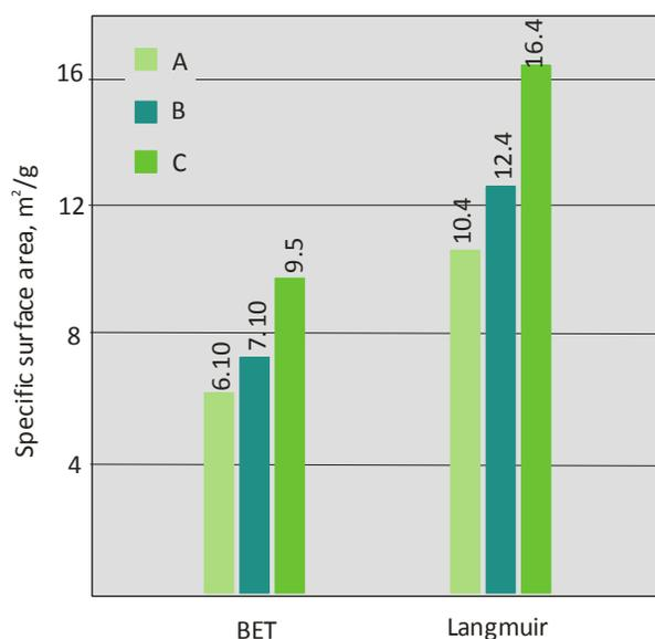
Fig. 16. BET and Langmuir specific surface area of PCL fibers with the molecular mass of  $M_w = 70,000-90,000$  g/mol obtained from 10% mixture of formic acid and hydrochloric acid with mass ratio of 70:30 with addition of  $\text{AgNO}_3$  with fraction of: A) 1%, B) 3%, C) 5%, after precipitation of silver with 2% ascorbic acid solution
