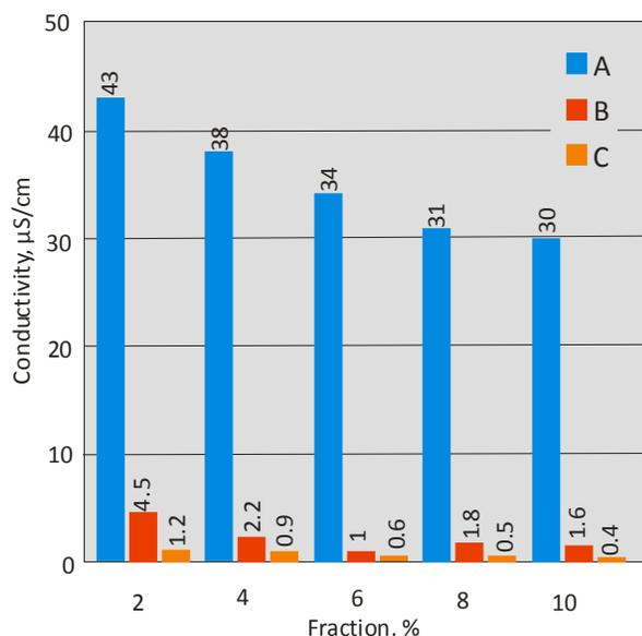
Fig. 7. Change of electric conductivity of polycaprolactone solution with fraction of 2-10% dissolved in mixture of hydrochloric acid and formic acid (A), chloroform and methanol (B) and a mixture of tetrahydrofuran and dimethyl sulfoxide (C)
