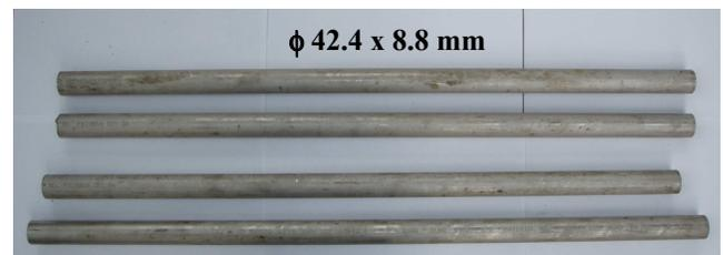
Fig. 2. Material for investigations in the form of the 4<sup>th</sup> stage steam superheater coils from Super 304H (X10CrNiCuNb18-9-3) steel
