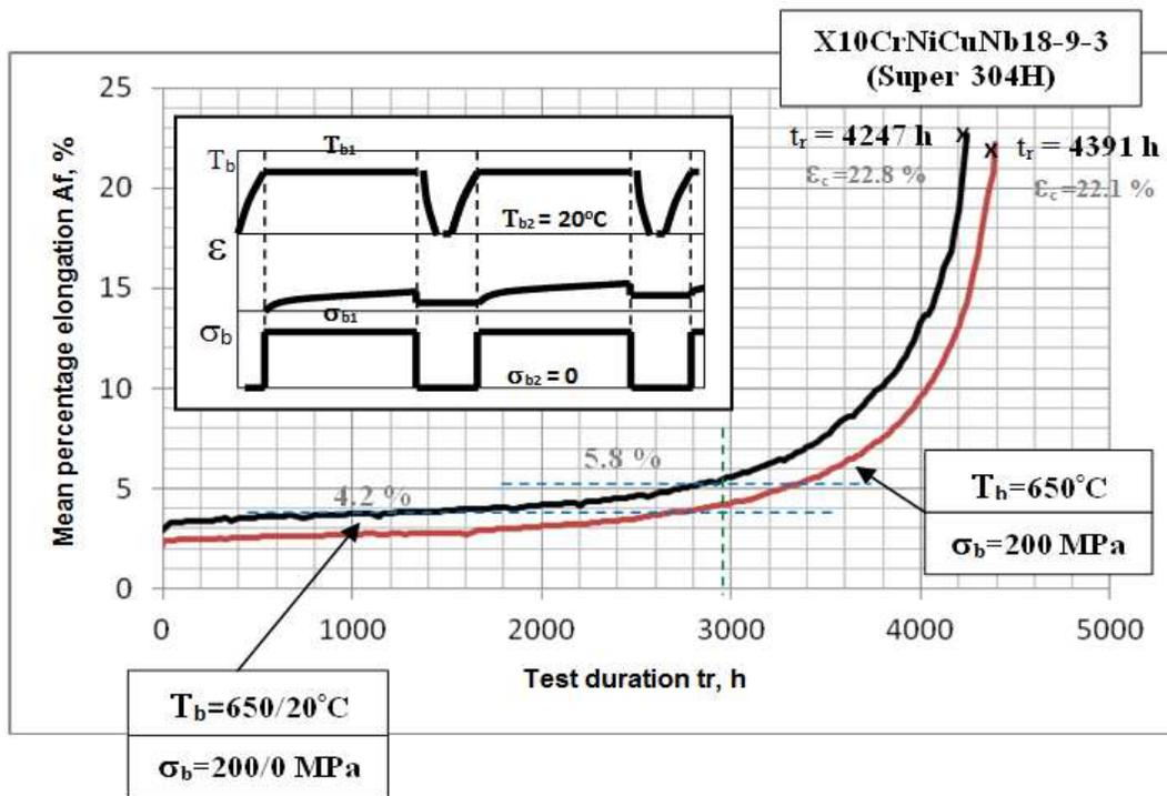
Fig. 4. Comparison of the results of creep tests conducted at cyclically changed test temperature  $T_b = 650/20^\circ\text{C}$  and constant test stress  $\sigma_b = 200/0$  MPa with the standard creep test ( $T_b = 650^\circ\text{C}$ ;  $\sigma_b = 100$  MPa)
