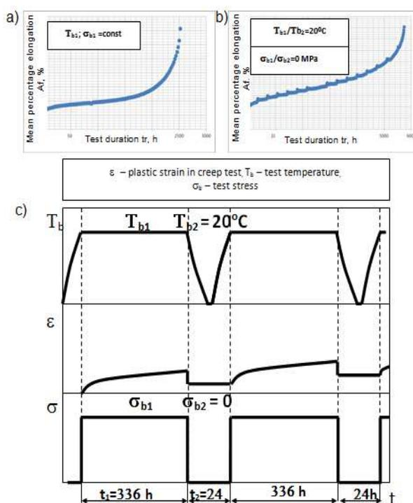
Fig. 3. Method for conducting creep tests: a) real standard creep curve for a test conducted at the constant test temperature and constant stress, b) real creep curve for a cyclic creep test conducted at cyclically changed temperature and with simultaneous stress relief, c) principles of cyclic changes in temperature  $T_{b1}/T_{b2}$  with simultaneous relief of stress  $\sigma_{b1}/\sigma_{b2}$  and recorded change in plastic strain  $\epsilon$  in completed cyclic creep tests (Fig. 3b)
