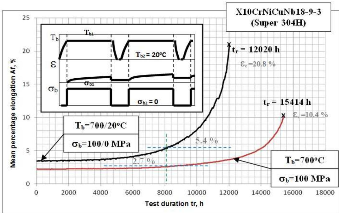
Fig. 5. Comparison of the results of creep tests conducted at cyclically changed test temperature  $T_b = 700/20^\circ\text{C}$  and constant test stress  $\sigma_b = 100/0$  MPa with the standard creep test ( $T_b = 700^\circ\text{C}$ ;  $\sigma_b = 100$  MPa)
