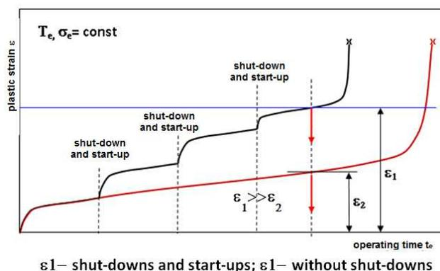
Fig. 6. Effect of shut-downs and start-ups on plastic strain due to creep
