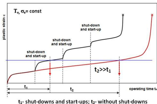
Fig. 7. Effect of shut-downs and start-ups on the time of reaching the same plastic strain
