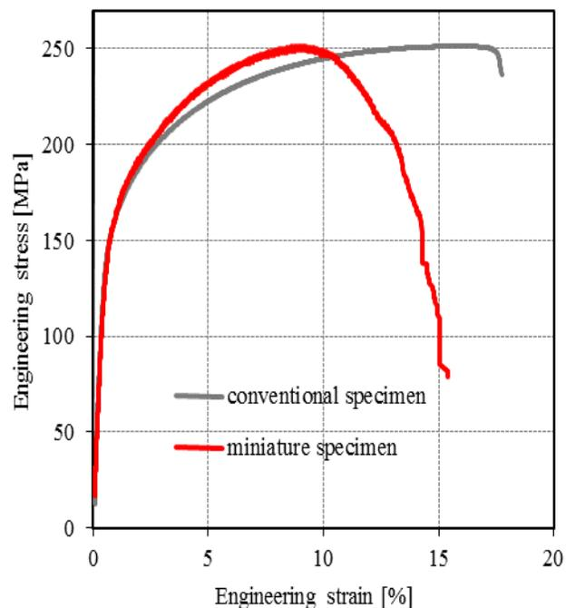
Fig. 5. Stress-strain curves of bulk material – miniature specimen compared to the conventional specimen.
