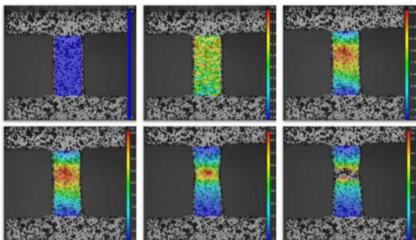
Fig. 3. Example of strain distribution in the specimen during the test
