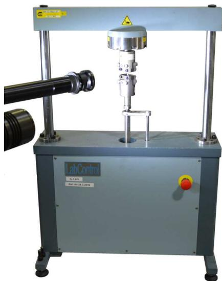
Fig. 4. The test setup for miniaturized tension
