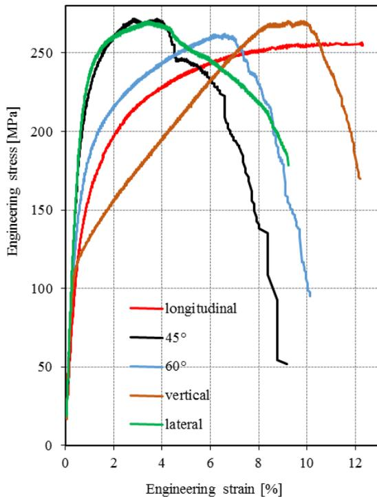
Fig. 6. Stress-strain curves of the miniature tensile specimens in various directions
