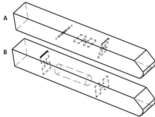
Fig. 1. ECAP billet with sampling scheme. Billet A contains tensile samples in longitudinal direction 45° angle from longitudinal direction and 60° to longitudinal direction. Billet B consists of tensile samples in vertical and lateral dimensions and sample for dilatometry
