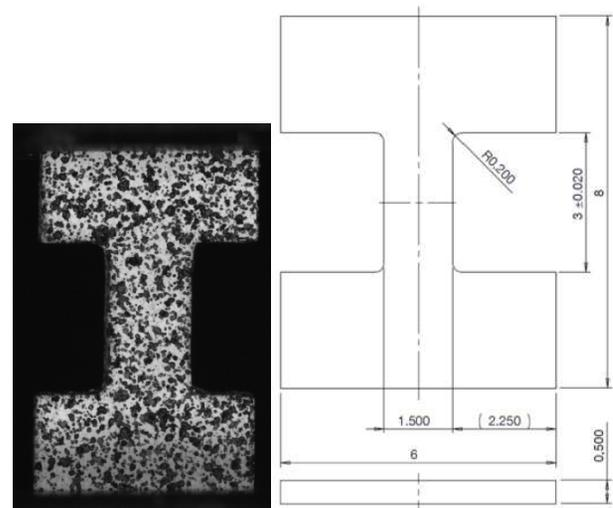
Fig. 2. Specimen with surface pattern and sample geometry
