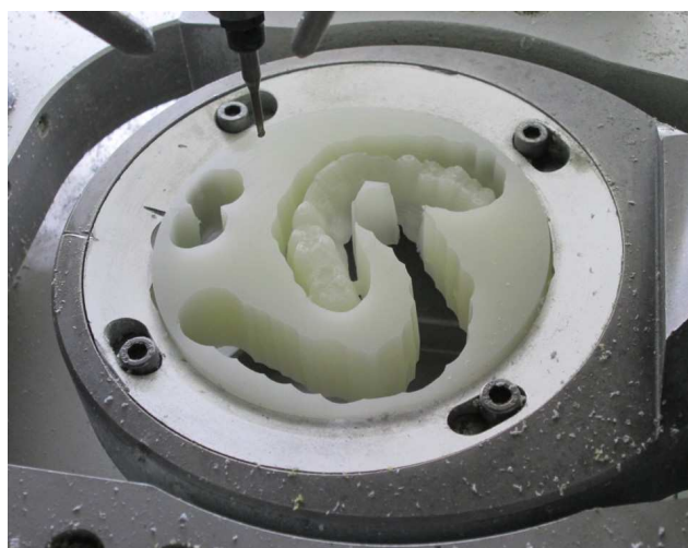
Fig. 15. Milling of the surgical guide in the CNC milling machine
