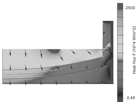
Fig. 4. Heat flux distribution for the furnace after several years of operation
