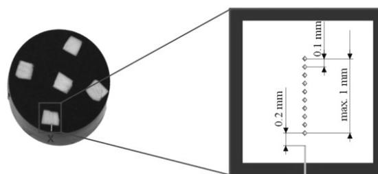
Fig. 4. Diagram of the microhardness indents scheme on the 5 x 5 mm bovine enamel specimens
